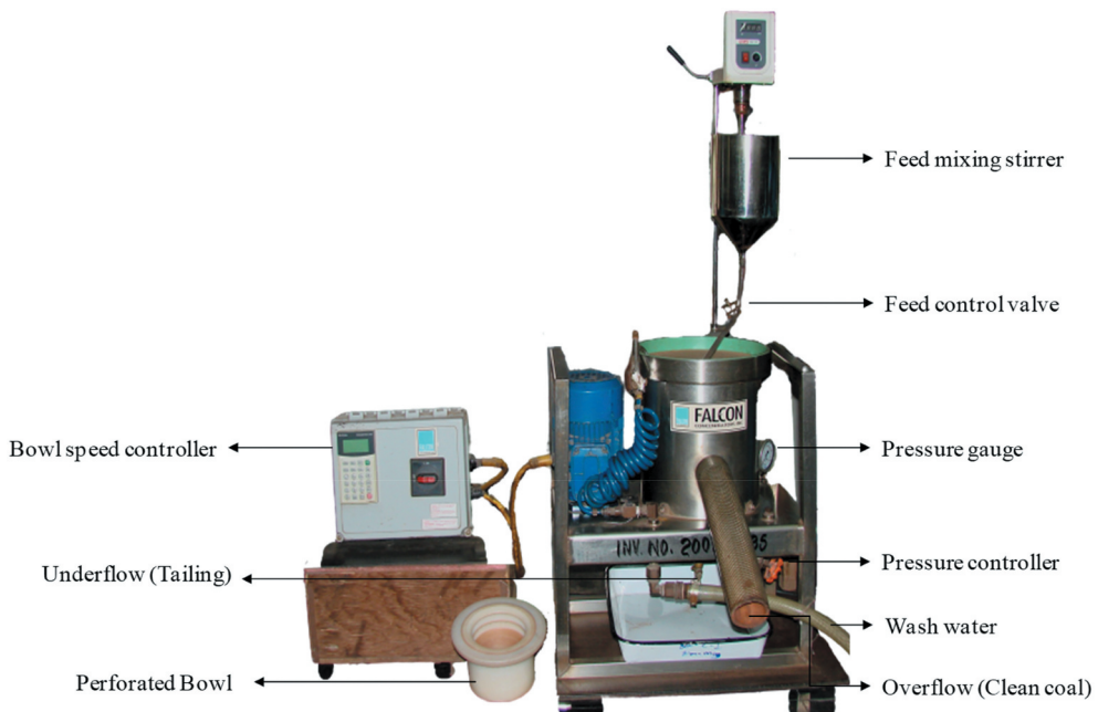
Figure 3. Schematic representation of Falcon SB40 concentrator.
