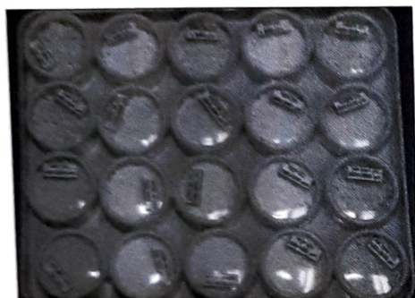
Fig. 5: Calcium phosphate (based on HAp and/or \beta -TCP) granules of various sizes for orthopaedic and dental filling
