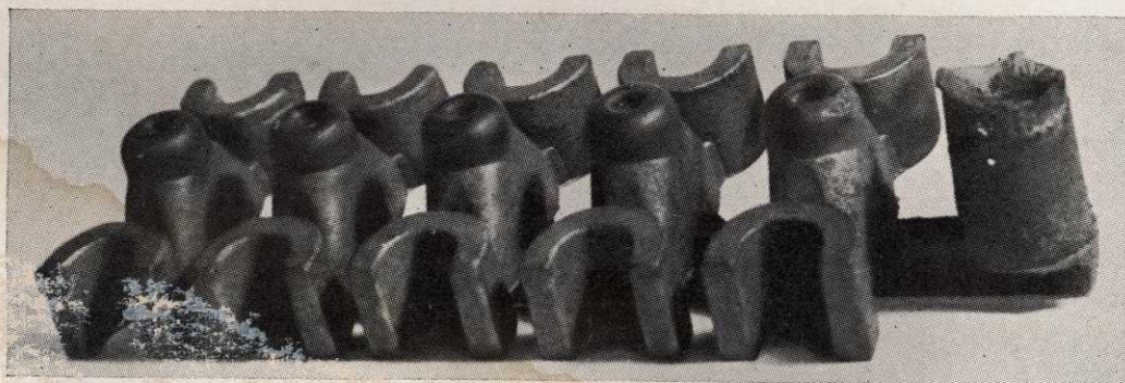
FIG. 27 — CASTINGS MADE BY SHELL MOULDING PROCESS
