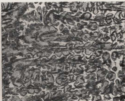
FIG. 30(a) — PHOTOMICROGRAPH OF ORIGINAL SAMPLE WITHOUT HEAT TREATMENT (Cu, 1.49 per cent) \times 240
