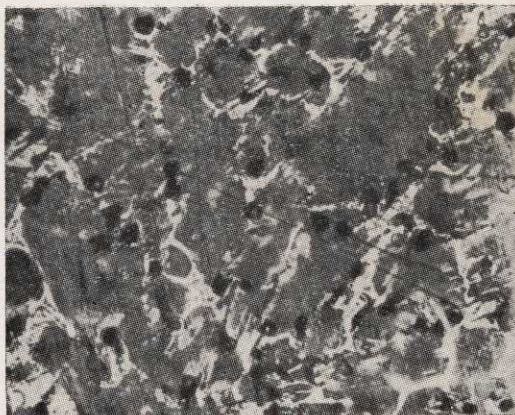
FIG. 29(a) — PHOTOMICROGRAPH OF ORIGINAL SAMPLE WITHOUT HEAT TREATMENT (Cu, 1.44 per cent) \times 240
