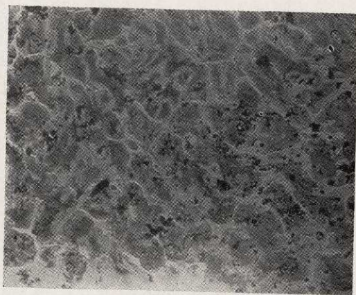
FIG. 31(a) — PHOTOMICROGRAPH OF ORIGINAL SAMPLE WITHOUT HEAT TREATMENT (Cu, 1.79 per cent) \times 240
