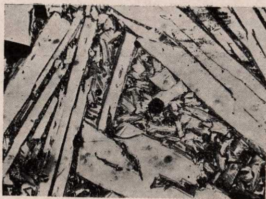
FIG. 48 — POLISHED SECTION OF BLAST FURNACE SLAG FROM TISCO SHOWING LATH-SHAPED CRYSTALS OF MELILITE
