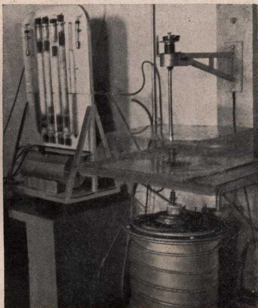
FIG. 16 — HIGH TEMPERATURE SLAG VISCOMETER, DESIGNED AND FABRICATED AT THE NATIONAL METALLURGICAL LABORATORY
