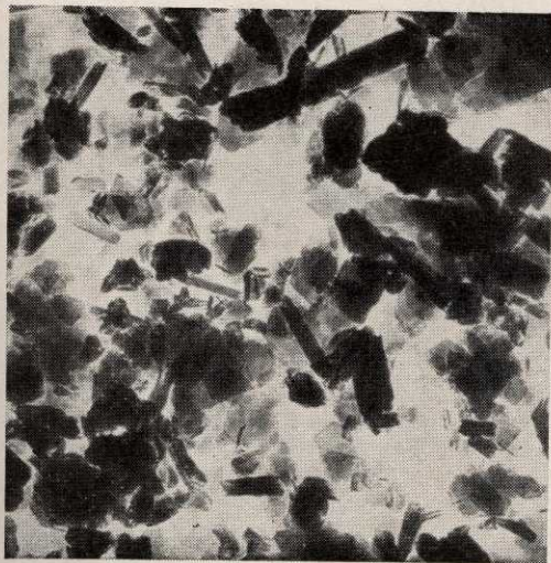
FIG. 55 — ELECTRON MICROGRAPH OF RAJMAHAL CHINA CLAY. \times 20,000
