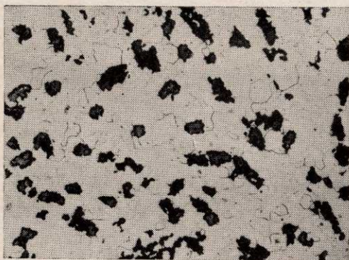
FIG. 31 — PHOTOMICROGRAPH OF CAST IRON INOCULATED WITH COPPER AND ANNEALED FOR 40 HR AT 850°C. \times 250
