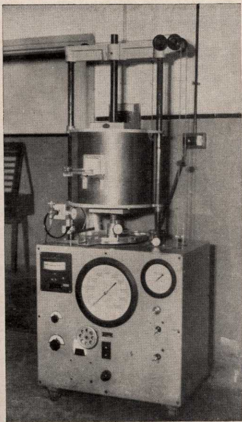
FIG. 29 — A VIEW OF THE APPARATUS FOR STUDYING THE PROPERTIES OF FOUNDRY MOULDING SANDS AT ELEVATED TEMPERATURES
