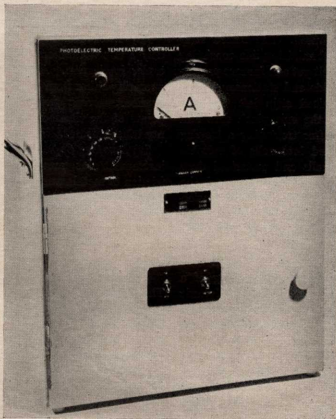
FIG. 78 — PHOTOELECTRIC TEMPERATURE CONTROLLER, DESIGNED AND FABRICATED AT THE NATIONAL METALLURGICAL LABORATORY
