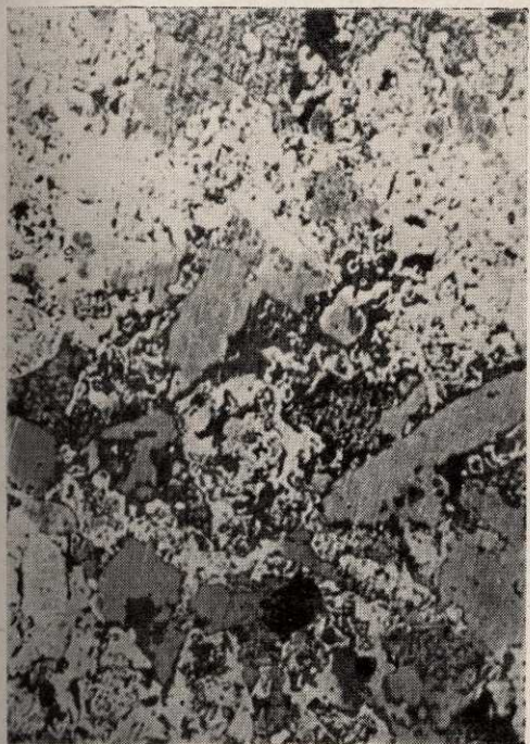
FIG. 21 — PHOTOMICROGRAPHS OF ALLOYS SINTERED AT 1200°C. \times 250
