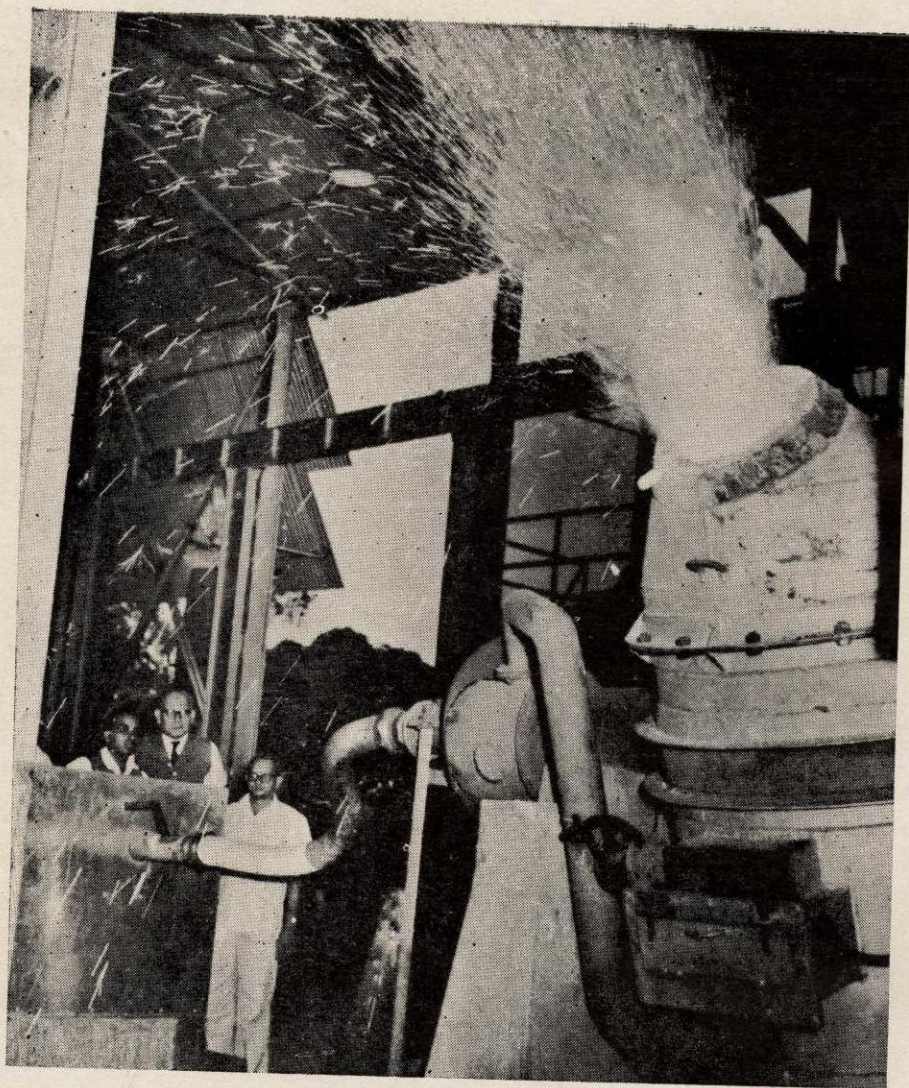
FIG. 66 — A VIEW OF THE SIDE-BLOWN BASIC CONVERTER OF \frac{1}{2} TON CAPACITY IN OPERATION. THE CONVERTER HAS BEEN DESIGNED AND FABRICATED AT THE NATIONAL METALLURGICAL LABORATORY
