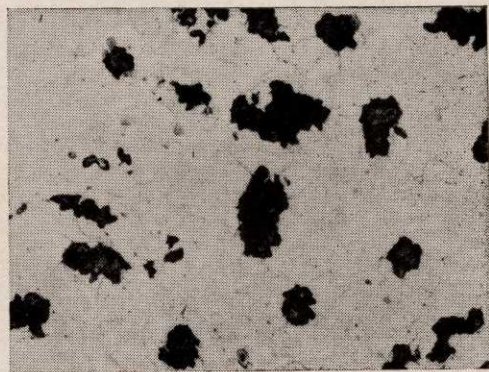
FIG. 32 — PHOTOMICROGRAPH OF CAST IRON INOCULATED WITH COPPER AND ANNEALED FOR 40 HR AT 850°C. \times 450
