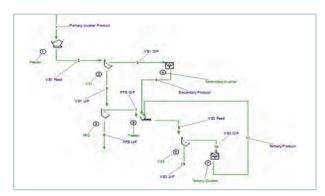
*Fig.12 : Crushing circuit under study.*
