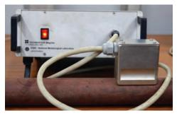
magnetization appears at the inner surface due to carburization during in-service operation in petrochemical industry. It can detect the presence of magnetic phase in non magnetic materials. The technology has been licensed for manufacturing to M/s Technofour, Pune.
