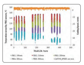
Fig.16: Real-Time Temperature monitoring using FBG
