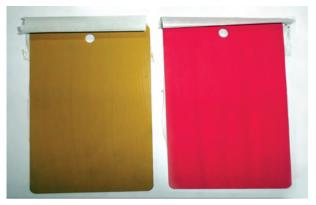
Fig. 8 : Developed paint using HPPI slag
