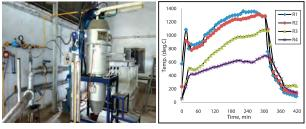
Fig. 5: Indigenously develope Stationary Bed Induration unit.
