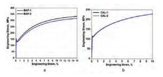
Fig.27: Stress-strain curves for Ti-Nb stabilized IFHS steel annealed after (a) batch annealing (BAF) and (b) continuous annealing (CAL) process showing the absence of Lüders elongation
