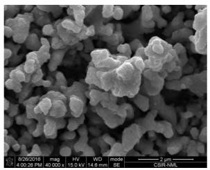
Fig. 1 : SEM of iron powder after reduction
