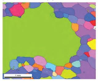
Fig.30 : Secondary recrystallized Goss grain obtained from a selection of suitable processing parameters
