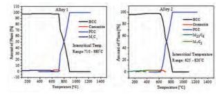
Fig.25:Thermodynamic property diagram showing the variation of phase fraction with temperature in Alloy 1 and Alloy 2
