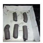
Fig. 4 : **a**. Extruding of fly ash-bottom ash mix in the ratio 1:1, with clay
