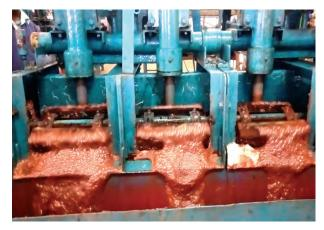
Fig.9: Pilot scale iron ore flotation study.
