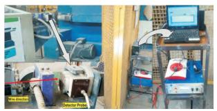
Fig.13 : Wire defect detection on-site.
