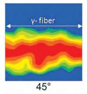
Fig.22: showing ODF section at  $\varphi_2 = 45^{\circ}$  on the RD-TD plane, of the optimized annealed cycle sample from GRADE A (B/N=0) illustrating fully developed  $\gamma$ -fibre beneficial for deep drawing
