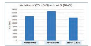
Fig.23 : Good combination of strength and ductility achieved in Grade B steel with (Nb+Si wt. %)=0.304
