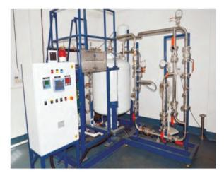
Fig. 7 : Closed loop corrosion test rig designed by CSIR - NML
