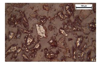
*Fig.8 : Photomicrograph showing locking of chromite with goethite, quartz and ferruginous clay.*
