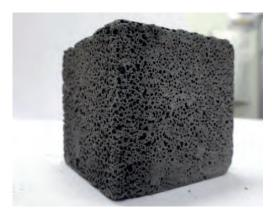
Fig. 7 : Developed porous sample using HPPI slag through geopolymerization
