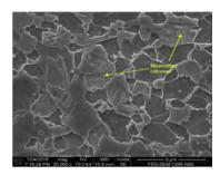
Fig.24 : Dual phase(DP) ferrite-martensite microstructure obtained in Grade C steel
