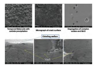
Fig.13: Micrographs revealing the summary of the failure investigation on front axle beam.
