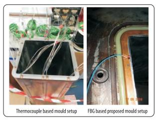
Fig.15: Temperature measurement conventionally, and using FBG
