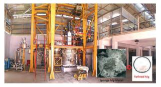
Fig. 2 : Pilot plant set-up along with the sample of sponge magnesium and the refined magnesium.
