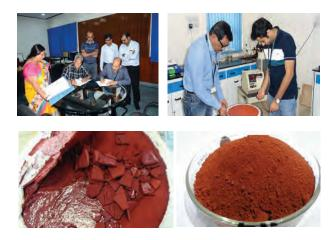
Fig. 13: : Iron oxide produced during demonstration of the process for production of red oxide pigment from chloride pickle liquor
