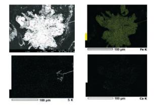
Fig. 10 : Back-scattered photomicrograph showing dendritic calcium siderite within the coal. Photographs represent the X-ray elemental mapping/distribution for Fe, S and Ca respectively
