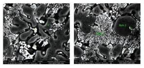
Fig.5: Microstructure of the Al-Si bracket containing eutectic Al-Si and alpha Al
