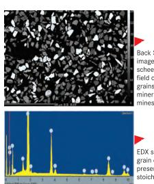
Back Scattered Electron image of only two scheelite grains in the field of view. Rest all the grains are gangue minerals present in the mines waste sample.
