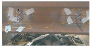
Fig.14: FBG sensor arrangement for strain measurement
