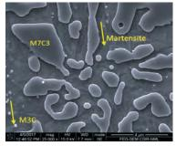
Fig.12: TEM image of cast iron having fine martensite (~3 nm),  $M_2C_3$  and  $M_3C$  phases
