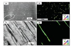
Fig.18 : EBSD analysis (a) secondary electron image; (b) corresponding inverse pole figure (IPF) of austenite phase; (c) image quality (IQ) map of high magnification scan and (d) corresponding IPF of austenite phase (green and black colors represent austenite and martensite phases, respectively)
