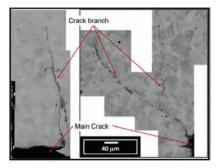
Fig.11: Cracking and crack branching in steel billets
