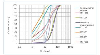
Fig.13 : Simulated particle size distribution of different streams.
