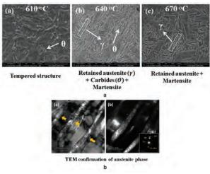
Fig.29: (a) SEM micrograph of the specimens annealed at different intercritical temperatures for 1 hour. (b) Bright field TEM micrograph showing retained austenite films (Left picture) indicated by arrows; Dark field TEM micrograph corresponding to the austenite diffraction spot (Right picture).
