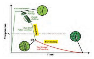
*Fig.17: Schematic of quenching and non-isothermal partitioning process*
