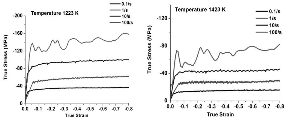
Fig. 7 : Effect of strain rate on flow stress at deformation temperatures of 1223 K and 1423 K
