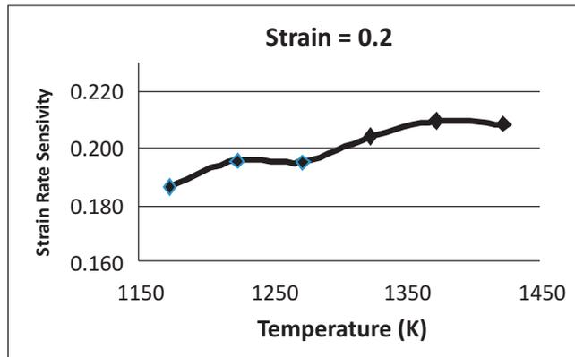
Fig. 9 : Variation of Strain Rate Sensitivity with Temperature
