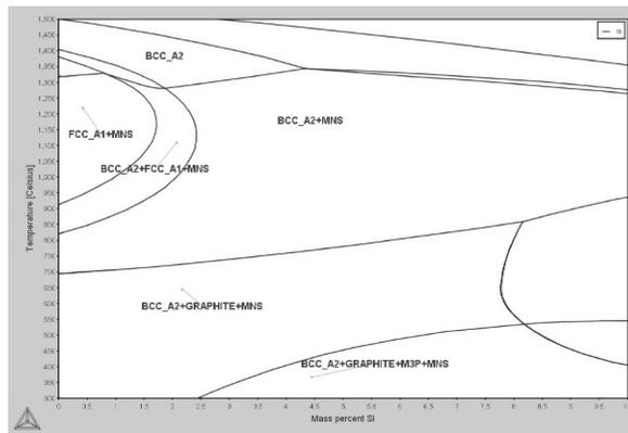
Fig. 1 : Phase Diagram as determined on ThermoCalc 3.1<sup>®</sup>
