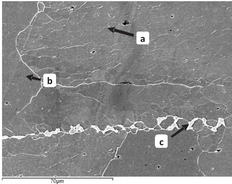
Fig. 4 : SEM Image showing: a) Strained grains, b) Unstrained grains and c) Second-phase
