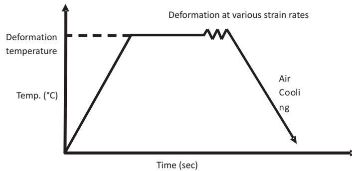
Fig. 2 : Hot Deformation Schematic
