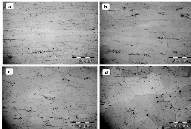
Fig. 3 : Optical Micrographs of Hot-Deformed Samples: a) 1223 K, 0.1/s, b) 1223 K, 10/sec, c) 1423 K, 0.1/s, d) 1423 K, 10/sec
