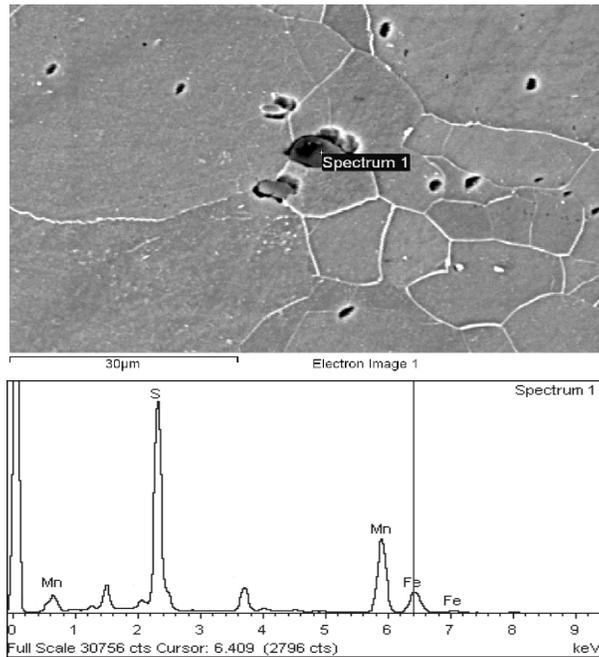
Fig. : 5 EDAX Analysis Showing Presence of MnS Precipitate
