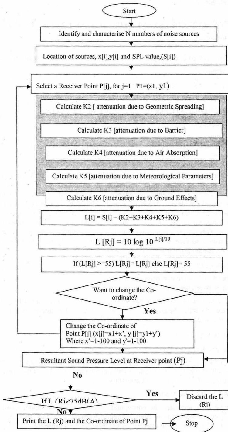
Fig. 4: Conceptual Flow Chart of the Model
