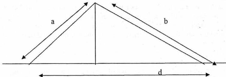
Fig. 3: Barrier Attenuation
