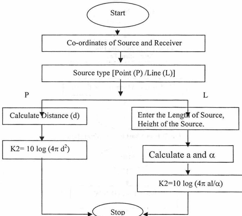
Fig. 5: Flow Chart- for Geometric Spreading
