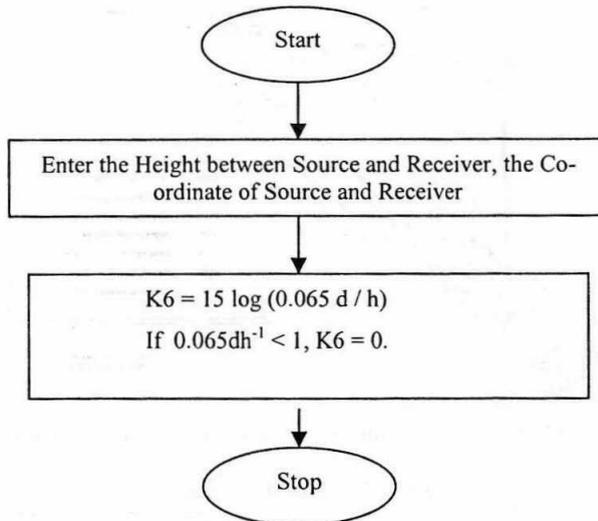
Fig. 9: Flow Chart for Ground Effect
