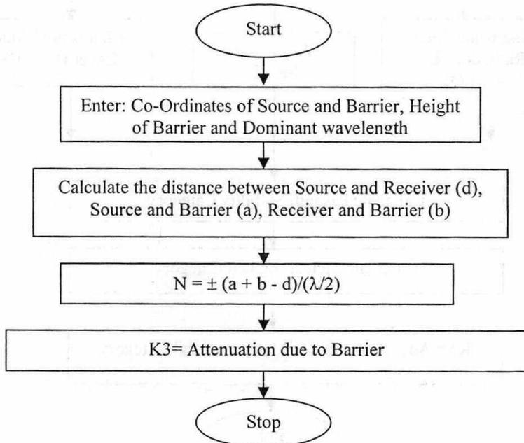
Fig. 6: Flow Chart -For Barrier Attenuation
