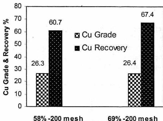
Fig. 3: Effect of Feed Particle Size
