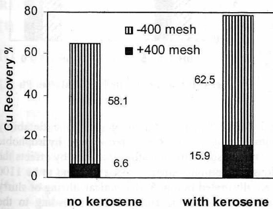
**Fig. 1: Effect of Kerosene**
