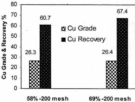
Fig. 3: Effect of Feed Particle Size
