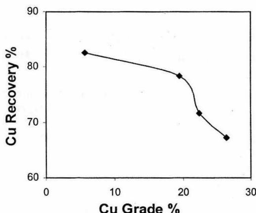
Fig. 6: Cu Grade Vs Recovery Curve
