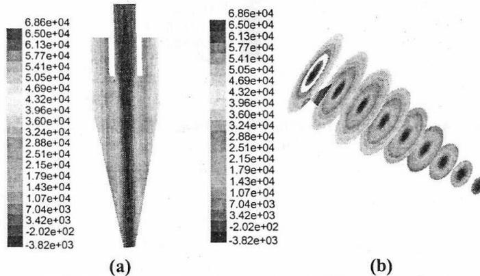
Fig. 6: (A) Contours of Static Pressure (Pascal) Along Vertical Plane, (B): Contours of Static Pressure (Pascal) Along Horizontal Planes
