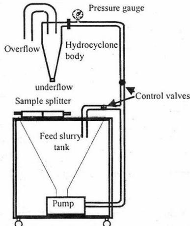
**Fig. 2: Hydrocyclone Experimental Test-Rig**
