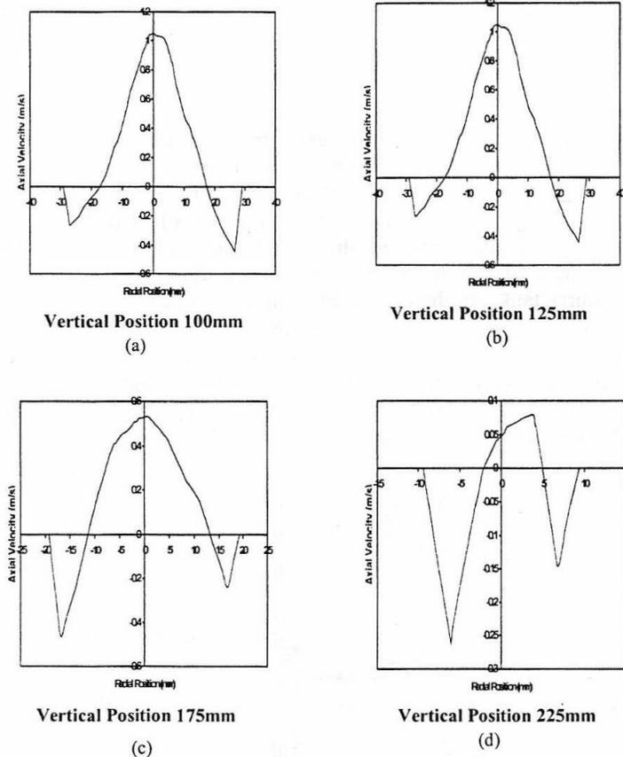
Fig. 3: Axial Velocity at Different Vertical Positions Inside the Cyclone
