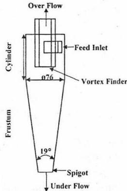
Fig. 1: Hydrocyclone Geometry
