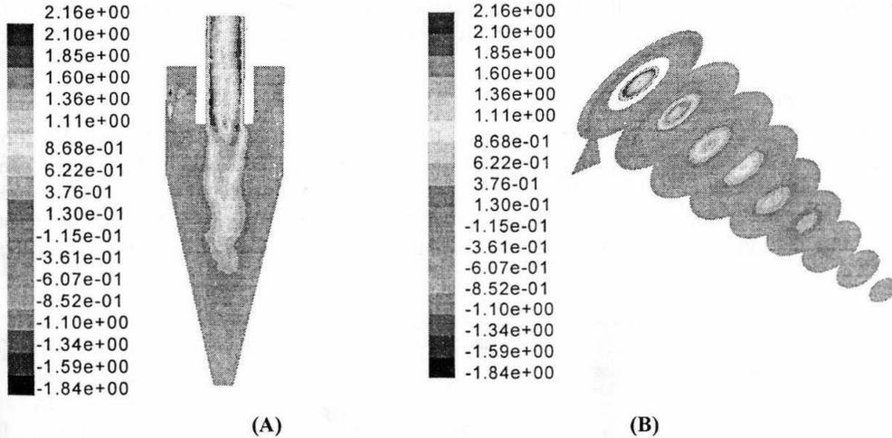
Fig. 4: (A) Contours of Axial Velocity (M/Sec) in Vertical Plane, (B) Contours of Axial Velocity (M/Sec) in Horizontal Planes
