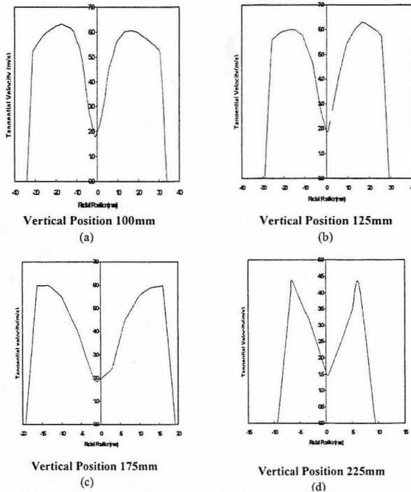
Fig. 5: Tangential Velocity at Different Vertical Positions Inside the Cyclone
