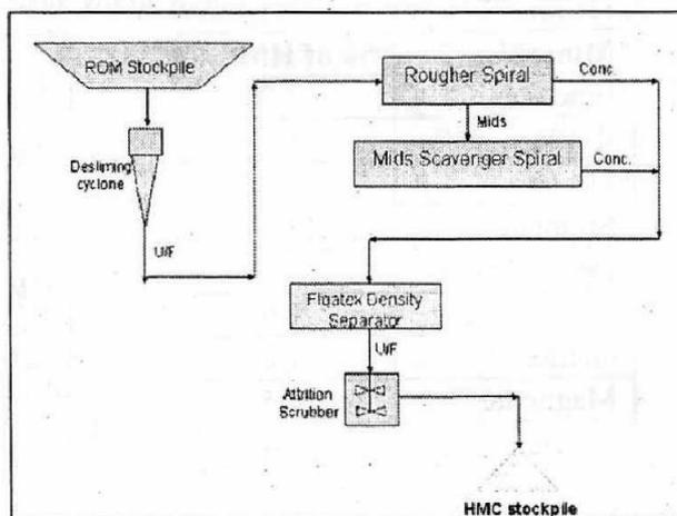
**Fig. 4: Primary Concentration Plant Flow Sheet using Spirals-Plus-Floatex Separator**
