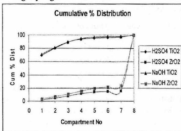
**Fig. 6: Cumulative Distribution of TiO<sub>2</sub> and ZrO<sub>2</sub> in Electrostatic Separation**
