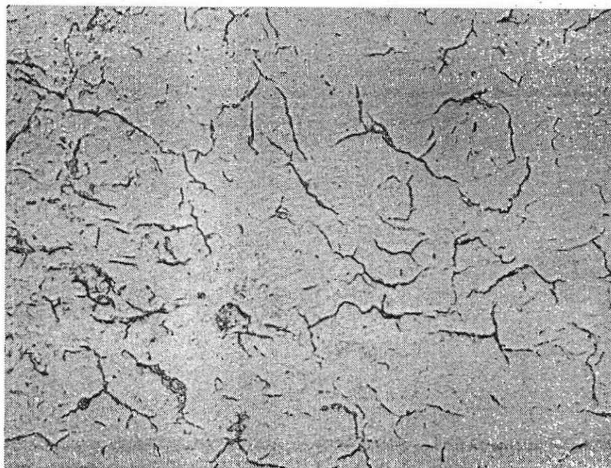
FIG. 1.VIII (continued) — MICRO-PHOTOGRAPHS OF DEPOSITED GAMMA MANGANESE DURING THE PERIOD OF TRANSFORMATION FROM GAMMA TO ALPHA MANGANESE
