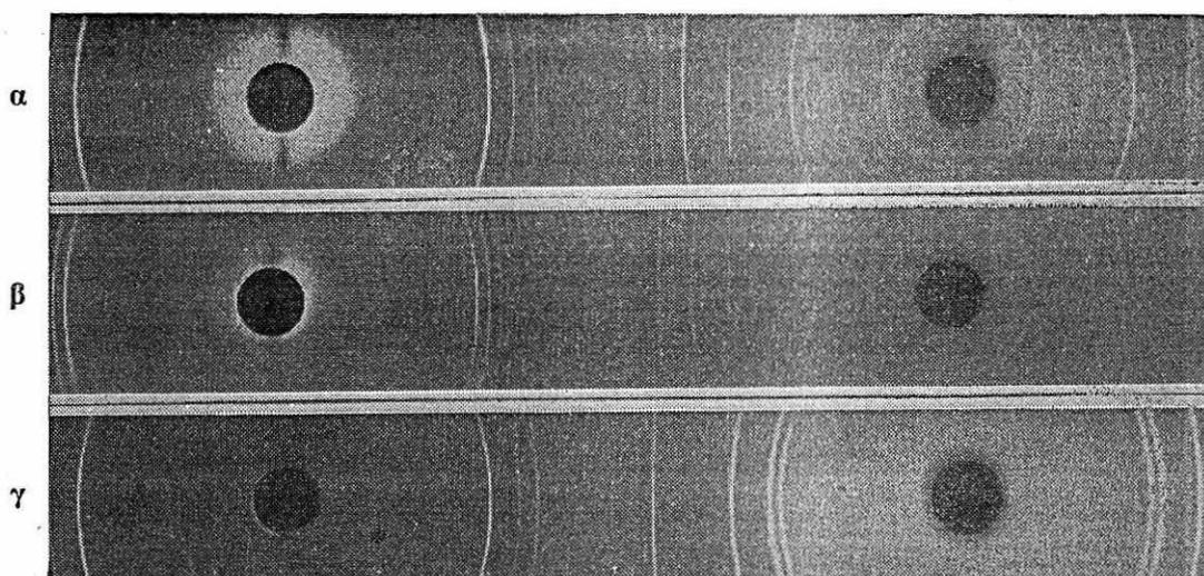
FIG. 1.II — X-RAY DIFFRACTION PATTERNS OF ALPHA, BETA AND ELECTRO-DEPOSITED GAMMA MANGANESE
