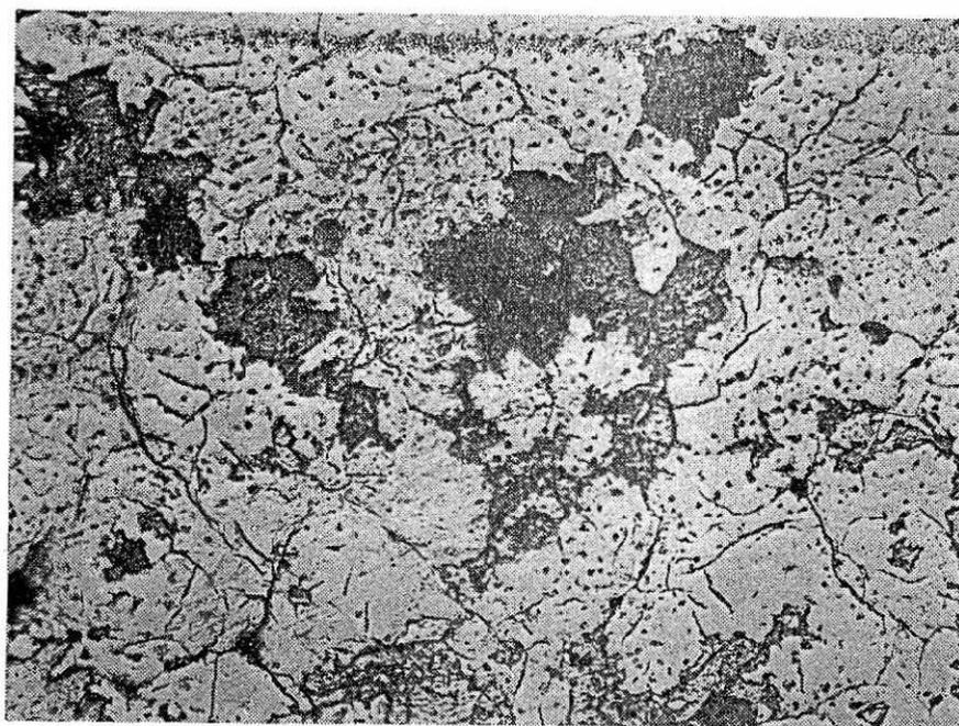
FIG. 1.VIII (continued) — MICRO-PHOTOGRAPHS OF DEPOSITED GAMMA MANGANESE DURING THE PERIOD OF TRANSFORMATION FROM GAMMA TO ALPHA MANGANESE
