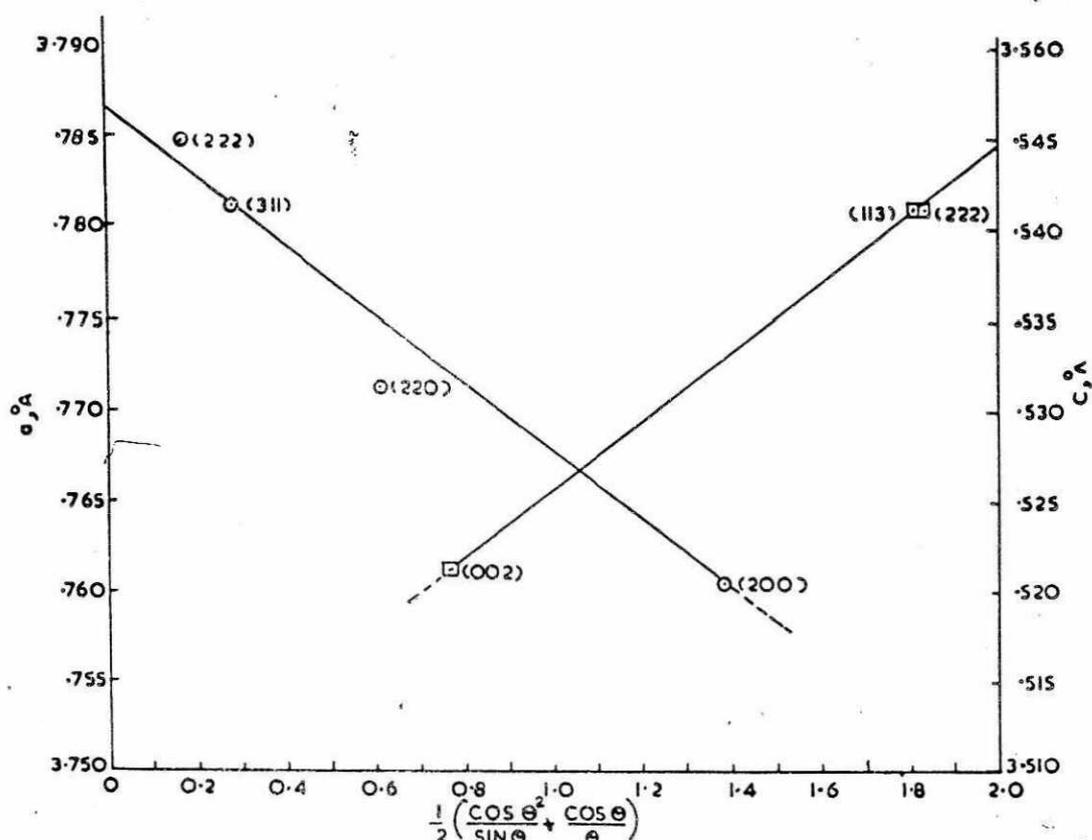
FIG. 1.V — EXTRAPOLATION OF 'a' AND 'c' OF ELECTRO-DEPOSITED GAMMA MANGANESE VS NELSON AND RILEY FUNCTION
