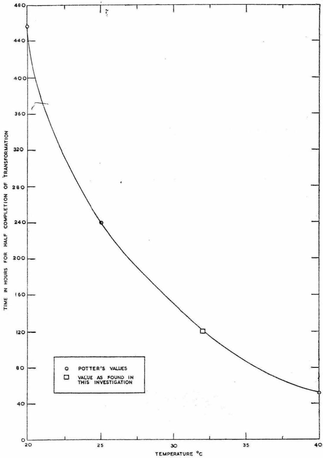
FIG. 1.VI — TIME FOR TRANSFORMATION OF GAMMA TO ALPHA MANGANESE VS TEMPERATURE
