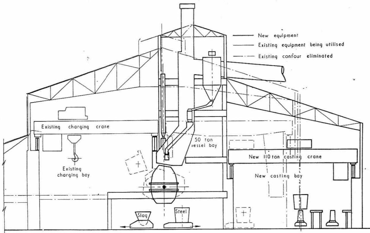
2 Typical cross-section through an integrated 50-ton LD vessel bay
