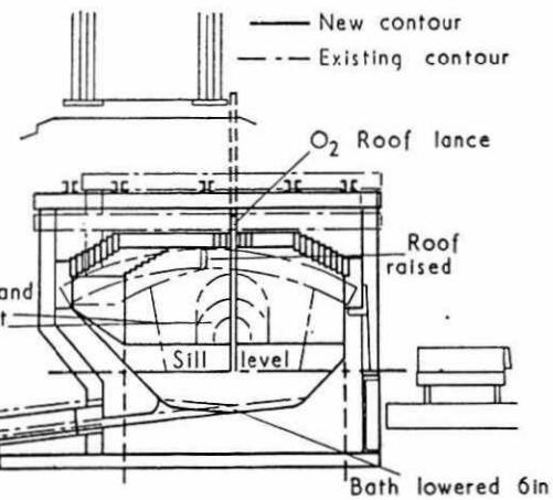
1 Typical cross-section through modified OH furnace
