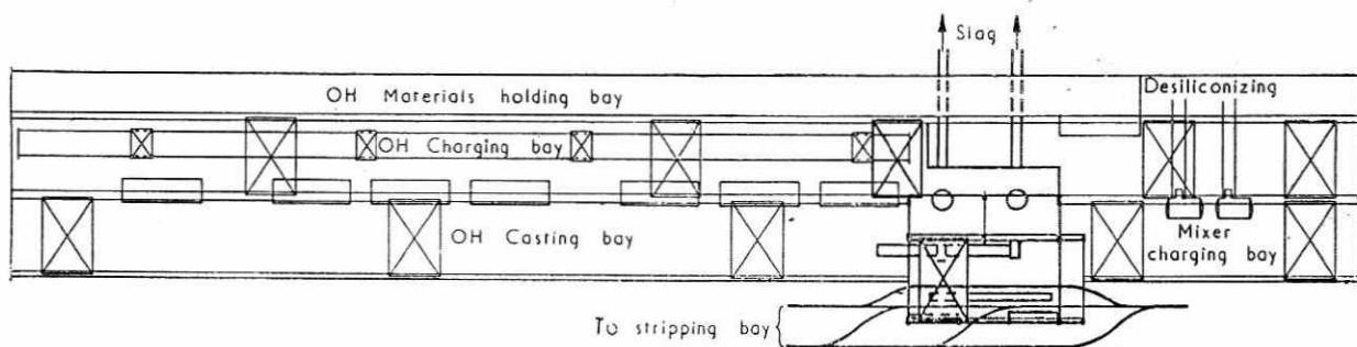
3 Typical layout of steelplant, showing integration of LD vessel
