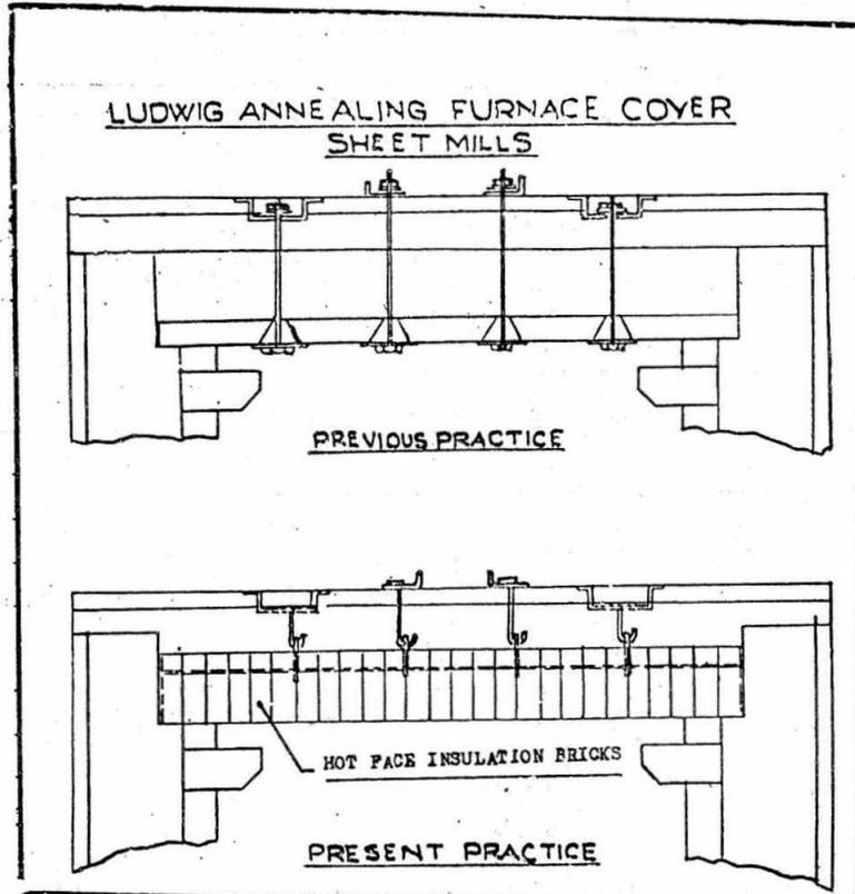
Fig. 3 Modification of furnace cover by replacing refractory tiles with hot face insulation.
