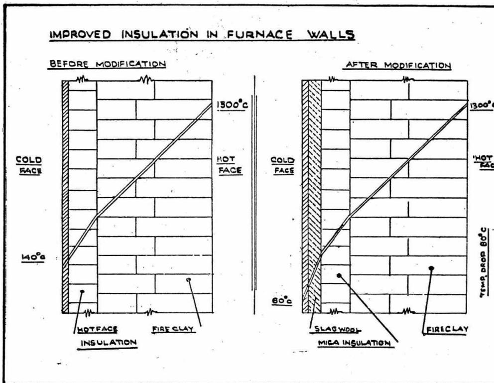
Fig. 5 Modified wall insulation.
