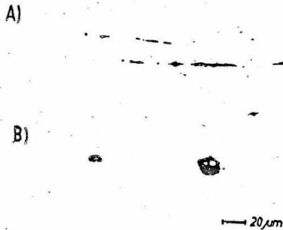
Fig. 9 A) Non-Metallic Inclusions in a 50-MM plate made of a Conventionally Molten Steel (Long Lines), and B) A Plate Made of a Steel Treated According to the TN Process (Globular Inclusions) 17)
