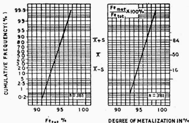
Fig. 9 Scattergram of Fe-contents and degree of metalization in metalized iron ore over 6 weeks of operation.
