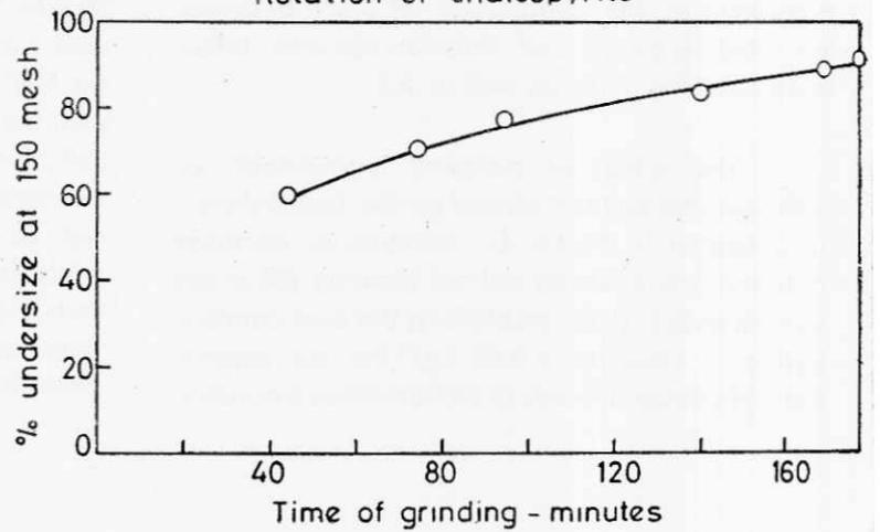
FIG 6. Effect of time on the production of -150 mesh ground ore.
