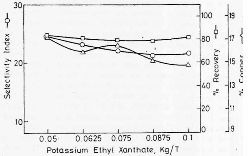
FIG 5 Effect of collector concentration on the flotation of chalcopyrite
