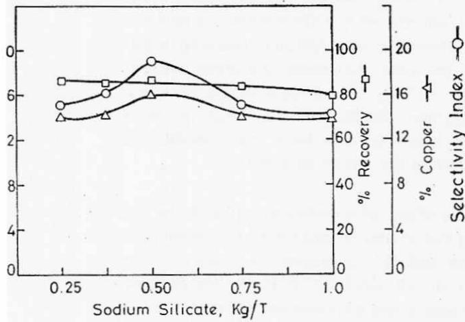
FIG 2 Effect of depressant concentration on the flotation of chalcopyrite
