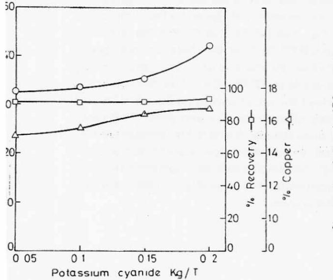
FIG 3 Effect of Potassium cyanide on the flotation of chalcopyrite
