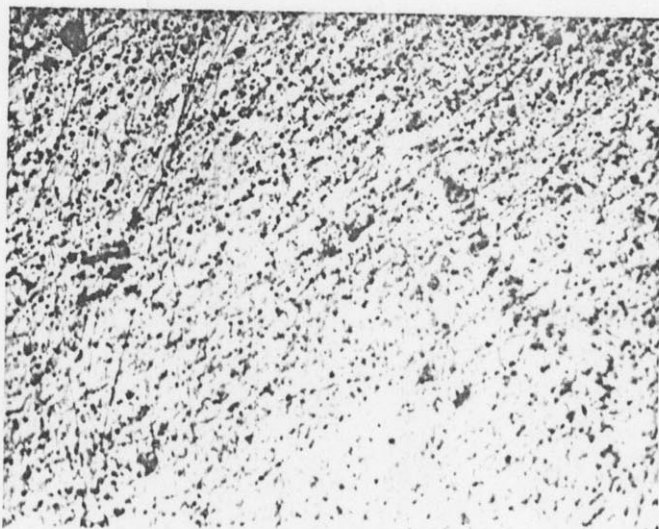
Fig.13. Optical photograph showing no crack in a film produced by the low chromium passivator having organic additives. (Galvasave treated, X 160, Unexposed).No cracking in the film is observed. This is due to the formation of amorphous type of coating which withstands compression.
