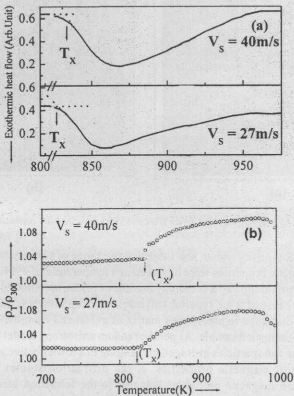
Fig. 2 : (a) DSC plots (b) Thermal electrical resistivity of ribbons prepared at different wheel velocities
