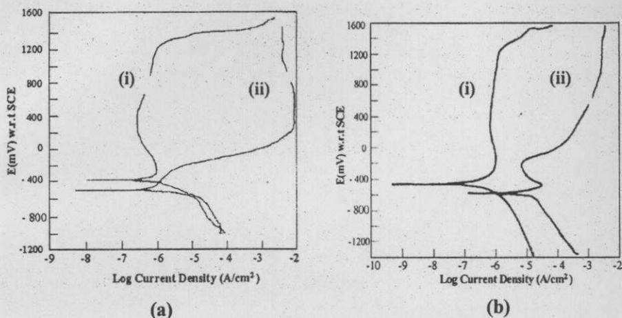
Fig. 4 : The potentiodynamic polarization plots of (a) as-cast and (b) heat-treated ribbon
