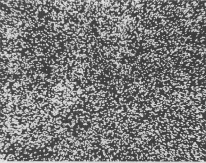
Fig. 2 : EPMA Ti dot mapping of  $(72\text{Ag}28\text{Cu})_3\text{Ti}$ , x400
