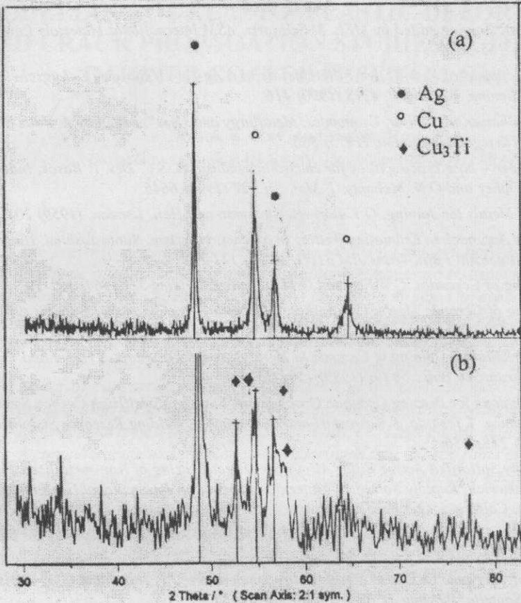
Fig.5 : X-ray diffraction of (a) 50Ag50Cu2Ti and (b) (50Ag50Cu)10Ti brazing alloys
