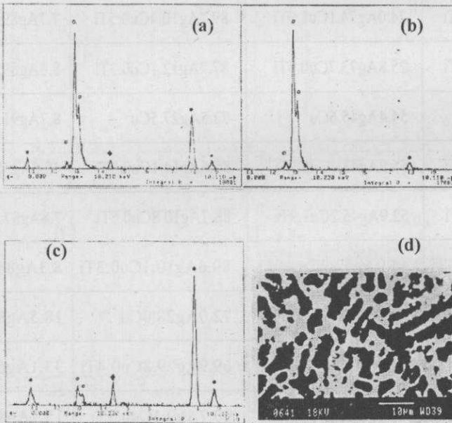
Fig.4 : EDX analyses of (50Ag50Cu)2Ti alloy, o – Ag, . - Cu and - Ti. (a) average, (b) at the silver rich bright phase (c) at the copper rich dark phase and (d) back scattered SEM image.
