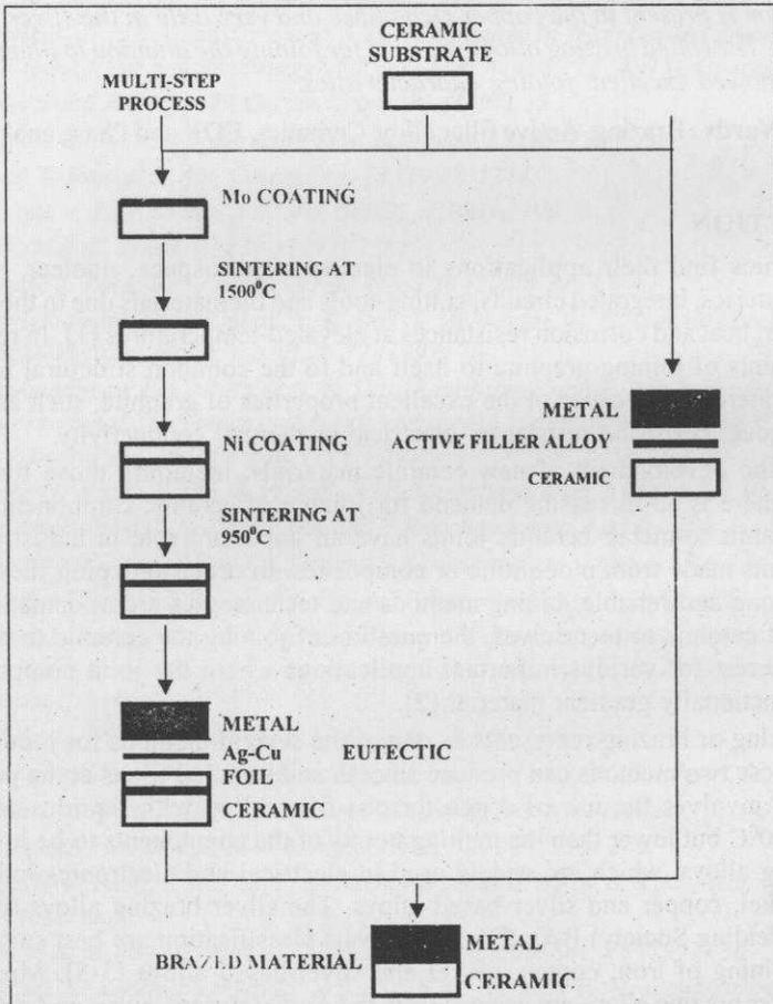
Fig. 1 : Methods of ceramic to metal joining
