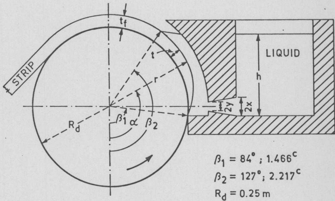
FIGURE 1 : Schematic representation of one roll strip caster
