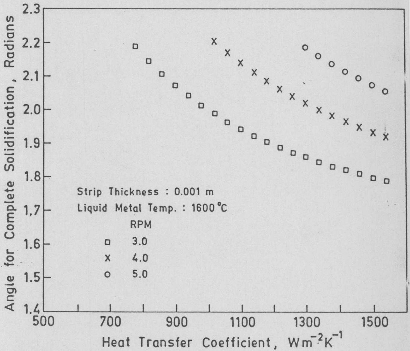
FIGURE 2 : Operating conditions required to produce a strip of thickness 0.001 metres
