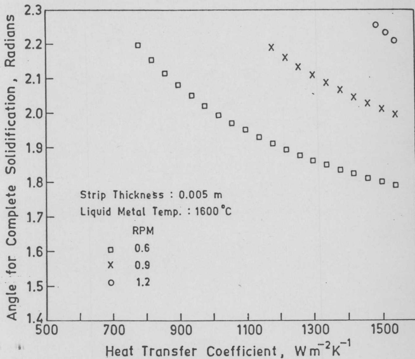
FIGURE 3 : Operating conditions required to produce a strip of thickness 0.005 metres
