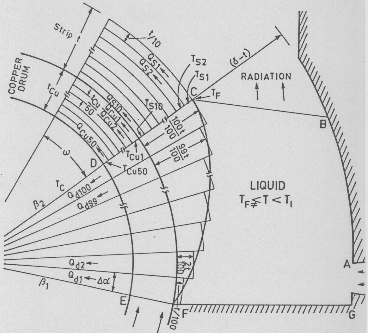
FIGURE 4 : Schematic representation of microscopic model based on enthalpy balance
