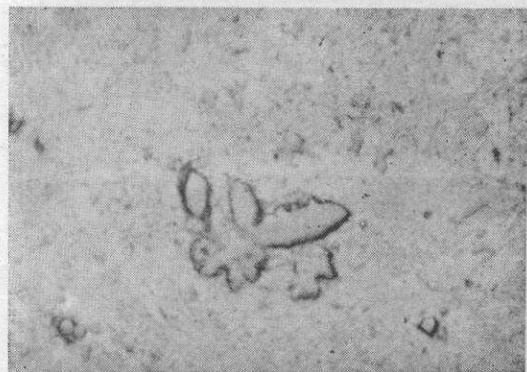
4 Sand cast sample, unetched ; showing coarse kappa \times 500
