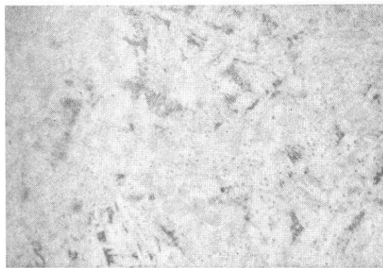
14 Sample from 600°C mold temperature, partly etched; showing dark rosettes \times 500
