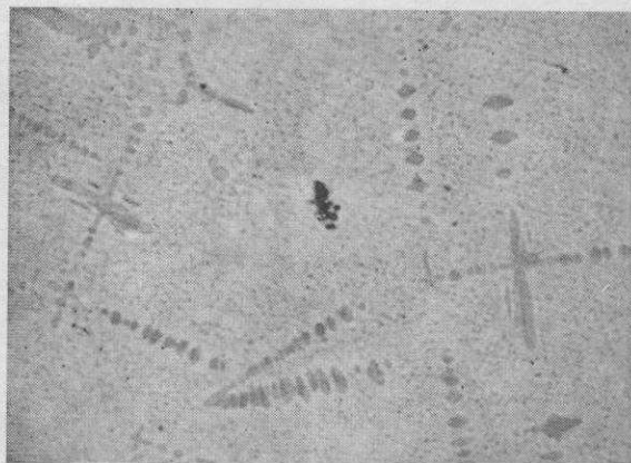
6 Sample from 1000°C mold temperature, unetched ; showing coarse and fine kappa \times 200
