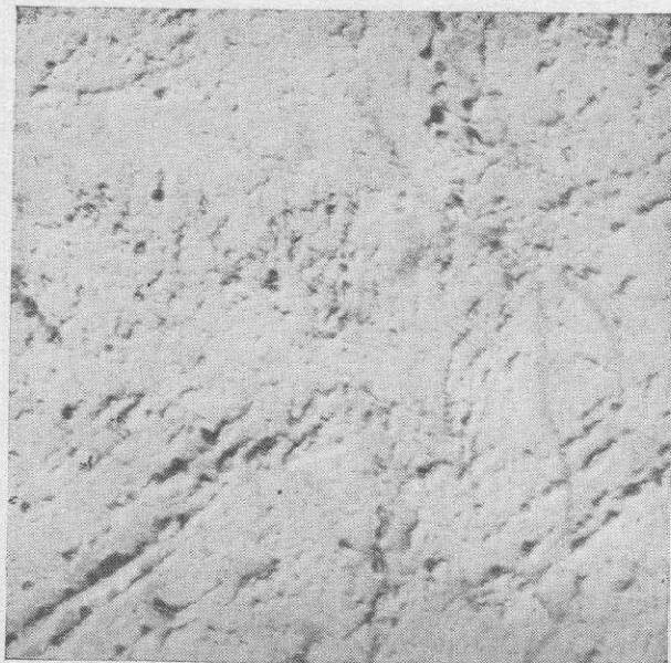
8 Stronger type carbides in sub-surface area of bearing track; Electron micrograph of C replica \times 22\,000
