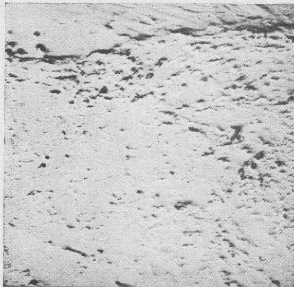
7 Transverse section through bearing track showing deformed metallographically changed surface material; Electron micrograph of C replica; Ni plated to protect edge during preparation \times 35\,000
