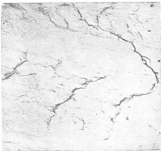
5 Transverse cracks in bearing surface ; Electron micrograph of C replica \times 19\,000
