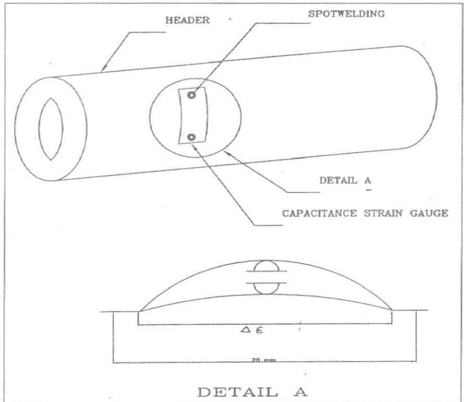
Fig. 1: A planer capacitance strain gauge
