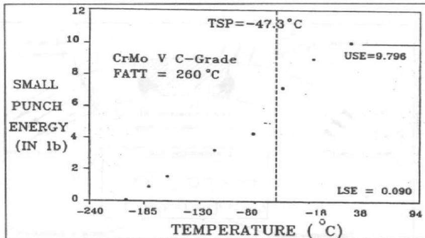
Fig. 3: Transition temperature,  $T_{sp}$
