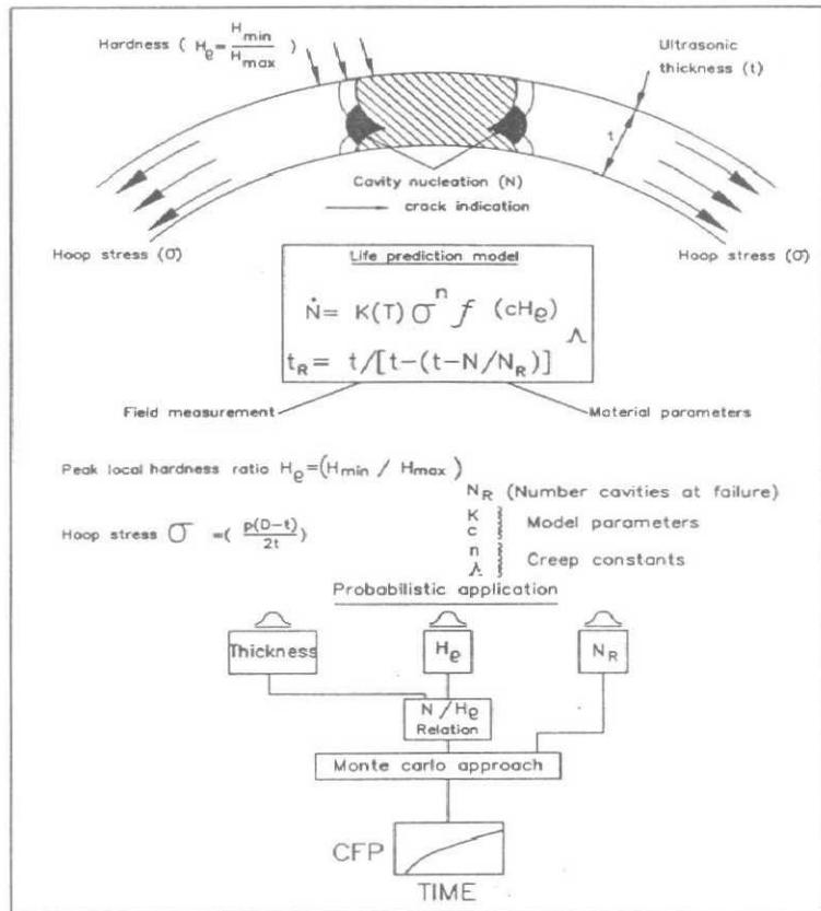
Fig. 4: Hardness difference method..
