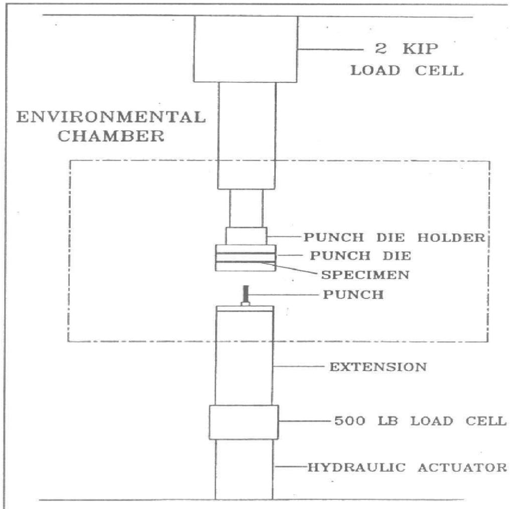
Fig. 2: Small punch test setup.
