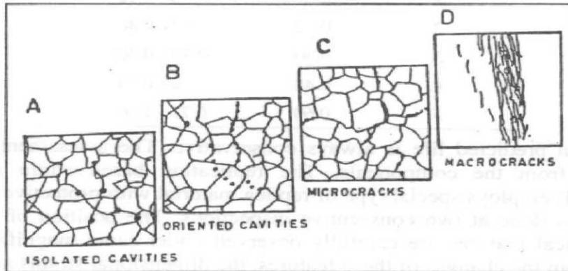
Fig. 5: Classification of creep damage.
