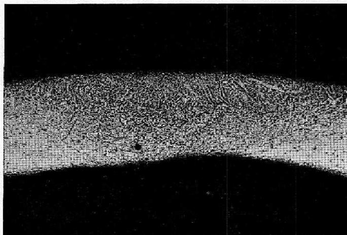
FIG. 10 (1198) — ATOMIC HYDROGEN WELD IN MONEL TUBE, COLD-DRAWN AND ANNEALED AFTER WELDING ( $\times 30$ )
