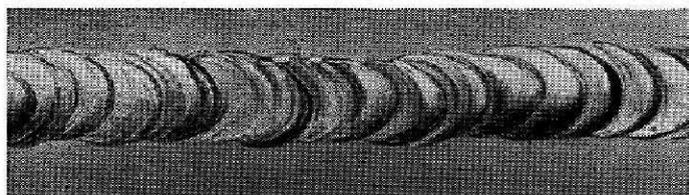
FIG. 9 — SURFACE OF ARGON ARC WELD IN MONEL USING INCO No. 60 FILLER WIRE ( $\times 2$ )
