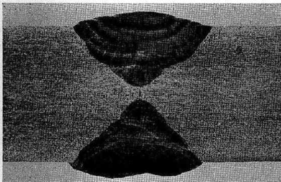
FIG. 7 (H. 2354) — MACRO-SECTION OF BUTT JOINT IN  $\frac{3}{8}$  IN. THICK MONEL PLATE. DOUBLE-VEE PREPARATION. LACK OF ROOT PENETRATION AT CENTRE OF JOINT (  $\times 3$  )
