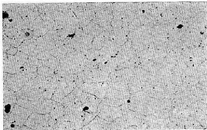
FIG. 2 — STRUCTURE OF K-MONEL AS SOLUTION TREATED AND AGED ( × 300 )
