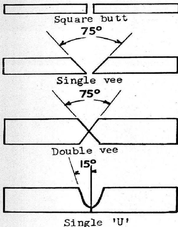
FIG. 3 — EDGE PREPARATION FOR VARIOUS THICKNESSES
