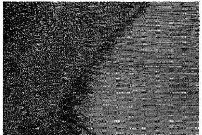
FIG. 6 (183) — WELD METAL AND ZONE OF PARTIAL FUSION IN METALLIC ARC WELD (× 50)
