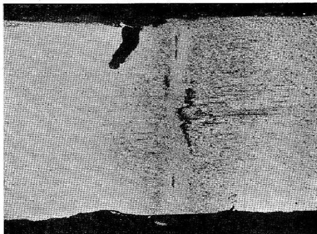
FIG. 16 — DEFECTS IN RESISTANCE BUTT WELDED MONEL PICKLING CHAIN SHOWING PIT ( $\times 6$ )
