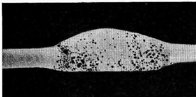
FIG. 8 (9534) — MACRO-SECTION OF ARGON ARC WELD IN MONEL, USING NORMAL MONEL AS FILLER WIRE ( $\times 10$ )
