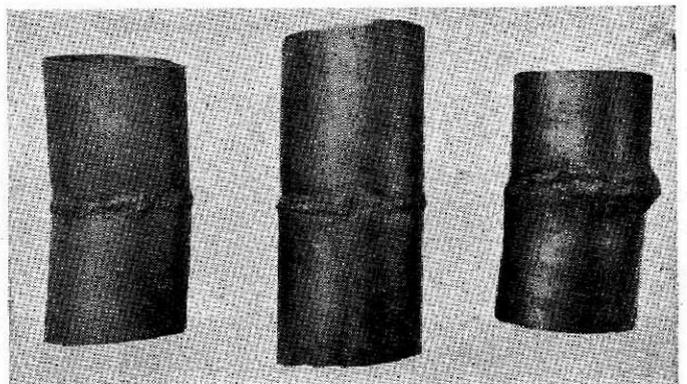
FIG. 19 — UNSOUND OXY-ACETYLENE WELDS IN MONEL TUBING, WHICH LED TO PITTING CORROSION ( $\times \frac{1}{2}$ )
