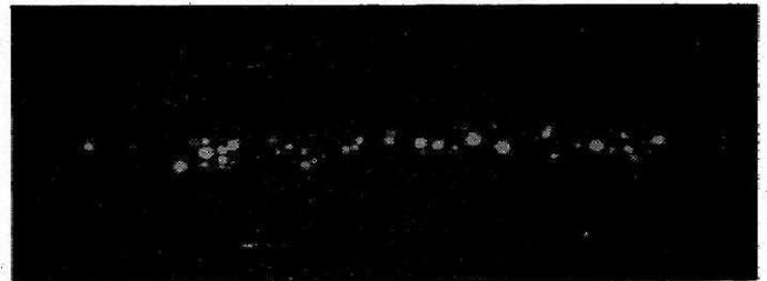
FIG. 5 — RADIOGRAPH OF UNSOUNDNESS IN MONEL ARC WELD RESULTING FROM USING DAMP ELECTRODES (× 1)
