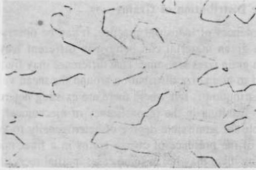
Fig. 6 : Tantalum sample polished and etched. Note lack of highly defined grain boundaries 600X
