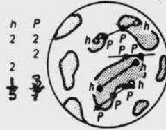
Fig. 2 : Chalkley method for determining the surface-to-volume ratio of discrete particles.
