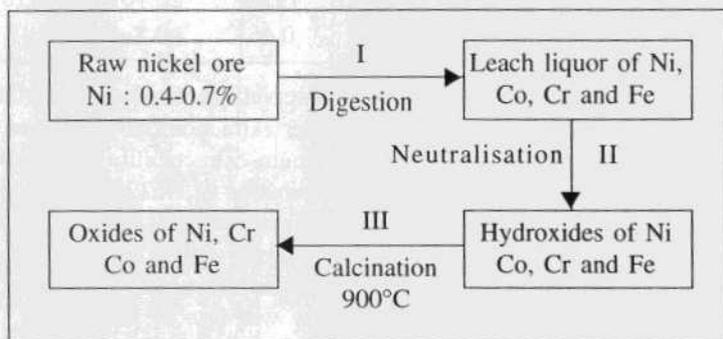
Fig.1 : Schematic diagram of the nickel enrichment scheme
