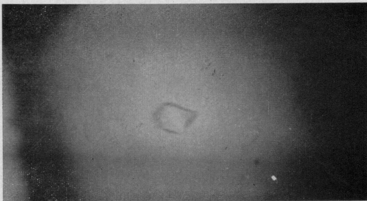
Fig. 16 Photomicrograph showing a primary spinel in high alumina blast furnace slag.
