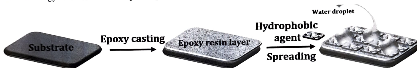
Fig. 2: Schematic representation of the synthesis procedure of epoxy superhydrophobic coating on various substrate
