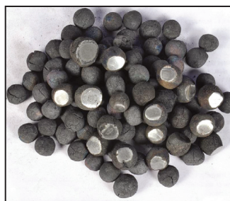
DRI from iron ore slime and middling coal
