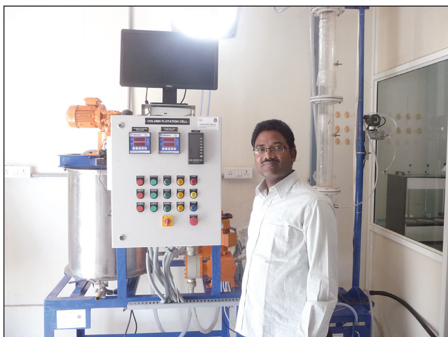
NML Flotation Column Lab Model installed at IIT Hyderabad for academic and R&D purpose
