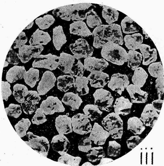
WASHED SAND GRAINS OF RAJMAHAL SILICA SAND RETAINED ON (i) 40 MESH ; (ii) 50 MESH ; (iii) 70 MESH ; AND (iv) 100 MESH ( \times 30 )
