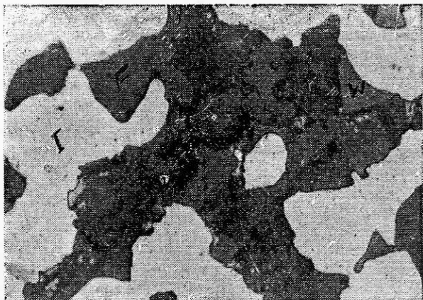
Fig 12 I = iron; W = wustite; F = fayalite C = iron cordierite
