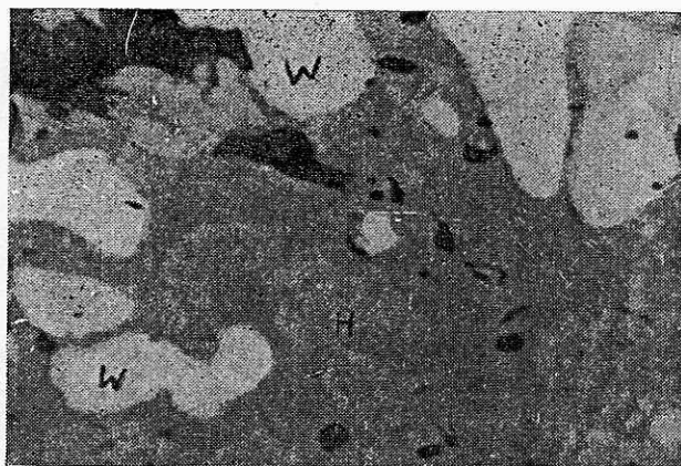
Fig. 9 Top fused layer in the zone 12 \frac{1}{2} to 14 \frac{1}{2} feet. F = fayalite H = hercynite; W = wustite. Dark areas are pores
