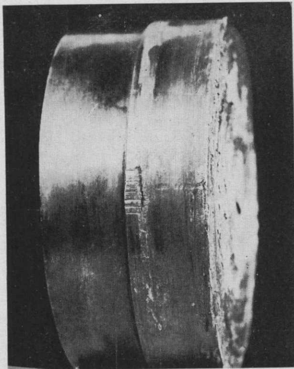
FIG. 3. Same as Fig. 2 taken from a side, showing Sharp Corner and poor surface finish
