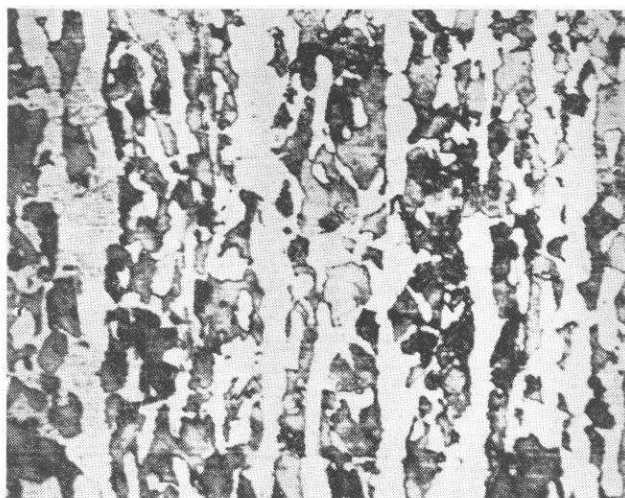
FIG. 5. Pronounced Banded structure of Steel I. Etched in Nital x-250.
