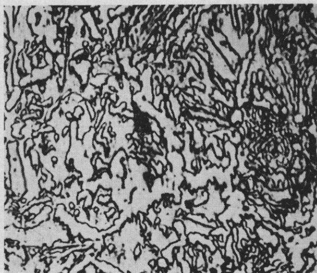
FIG. 9. Highly Abnormal Structure of Steel I on pack carburisation. Etched in Nital x-1200.
