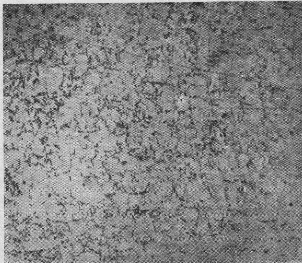
FIG. 7 McQuaid Ehn Grain-size No. 7-8 of Steel I. Etched in Sodium Picrate x-100.
