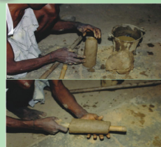
Traditional method of tuyere making
