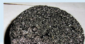
BLENDED COKE AKHURUSHABA COAL 70% KONYA COAL 30% HTC AT 850°C
