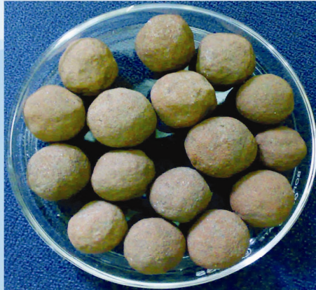
FIG. 1: COLD BONDED IRON ORE PELLETS (PREPARED FROM 'BLUE DUST' OF HIGH IRON CONTENT)
