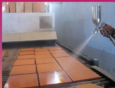
Titania coating on terracotta tiles (Pilot trials)
