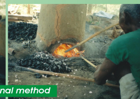
Fused mass of iron with slag
