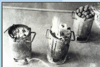
BLENDED COKE AKHURUSHABA COAL 70% KONYA COAL 30% HTC AT 750°C
