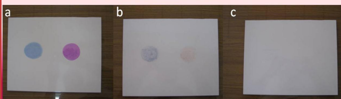
Patches of standard dye methylene blue and rhodamine 6G on the coated tile (a) before exposure (b) after 1h exposure (c) after 2 h exposure, to sunlight.
