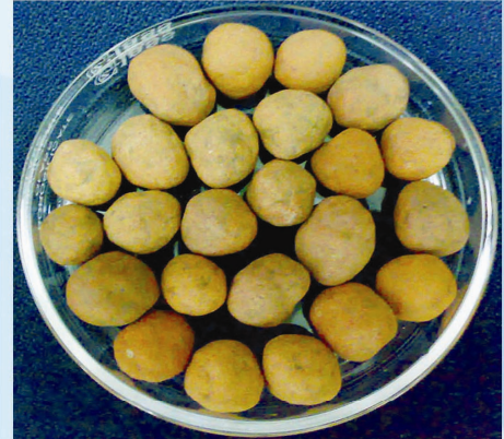
FIG. 2: COLD BONDED IRON ORE PELLETS (PREPARED FROM 'ORE HAVING MODERATE IRON CONTENT')
