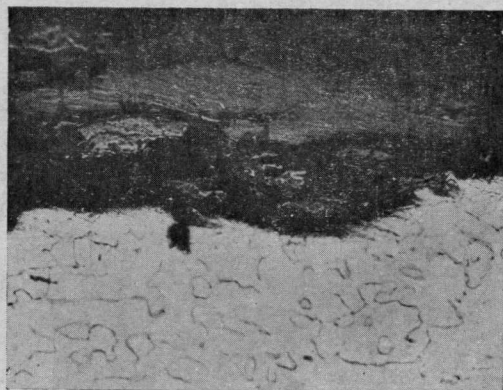
FIG. 54 — MICROSTRUCTURE OF EXPOSED GALVANIZED M.S. WIRE SHOWING ONLY CORROSION PRODUCT OVER THE BASIS METAL. ETCHED IN NITAL \times 450
