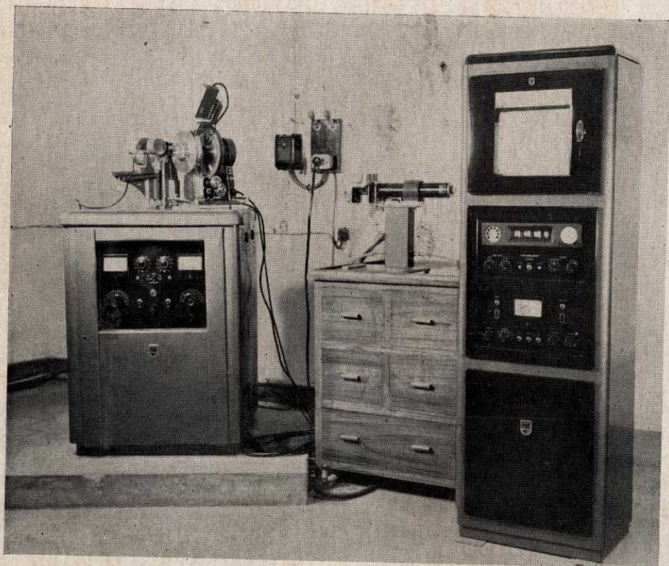
FIG. 4 — A VIEW OF THE PHILLIPS X-RAY DIFFRACTION UNIT, DIFFRACTOMETER WITH GEIGER-MÜLLER COUNTER AND RECORDER. X-RAY SPECTROGRAPH ATTACHMENT SHOWN AT THE CENTRE TABLE
