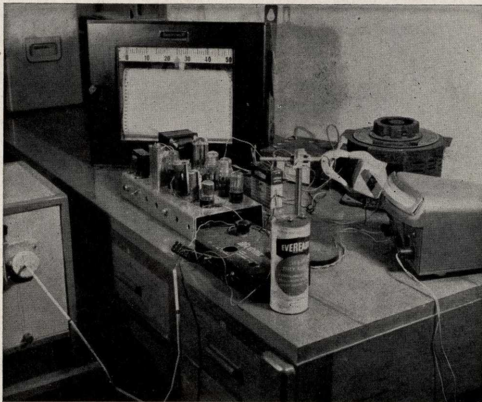
FIG. 28 — PHOTOELECTRIC TEMPERATURE CONTROLLER DESIGNED AND FABRICATED AT THE NATIONAL METALLURGICAL LABORATORY
