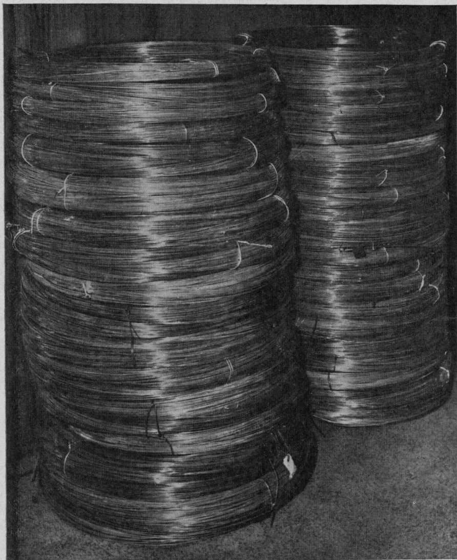
A typical heap of PM-2 aluminium Cables developed at NML produced on semi-commercial scale in an aluminium plant.
