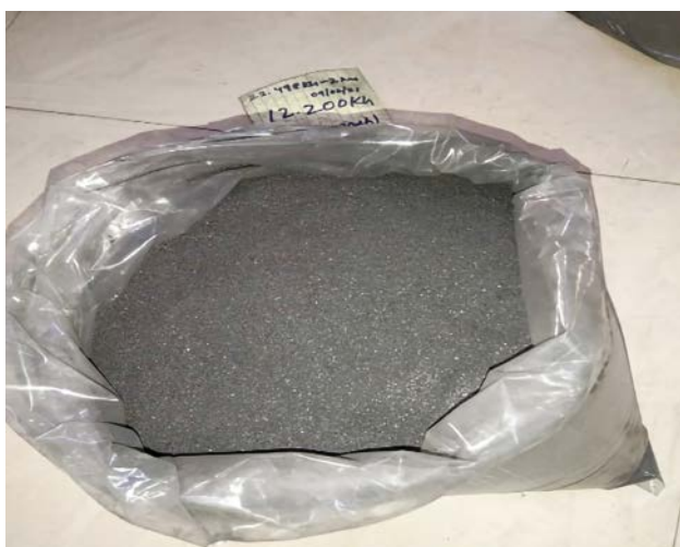
Figure 5: The dried, pulverized and screened slag sample to be used for alkali roasting
