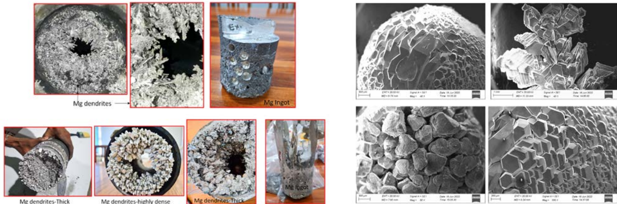
Figure 10. Morphologies of Mg distillates in various shapes and sizes with SEM micrographs of dendritic and spherical droplet deposits during condensation
