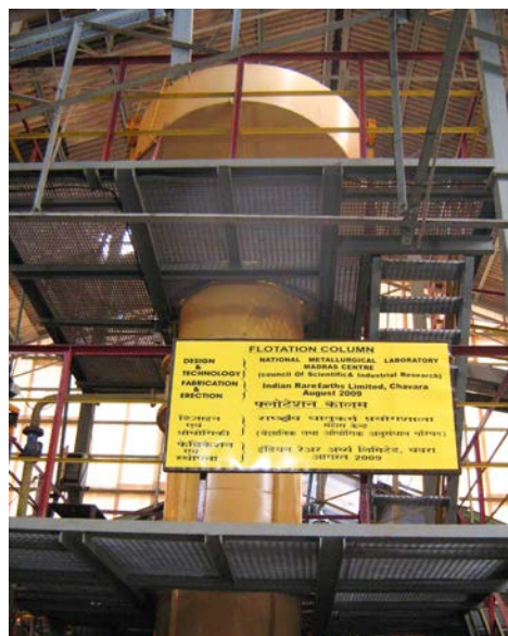
Figure 8: 150 tonnes per day commercial-scale flotation column at M/s IREL, Chavara, Kerala
