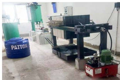
100l Black Mass Leaching Facility
