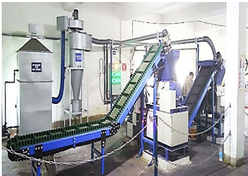
CSIR's First Battery Dismantling &amp; Black Mass Retrieval Facility (1TPD)
