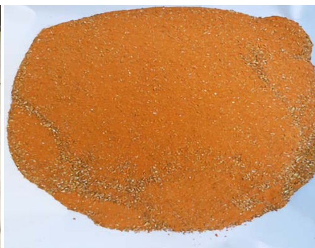
Figure 6: Ammonium Meta-Vanadate produced from coal-slag.
