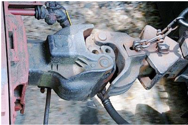
Figure 1: (a) Centre Buffer Coupler (CBC) joining two rolling stocks; (b) Different parts of CBC (Yoke, Body, Knuckle)
