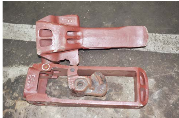
Figure 1: (a) Centre Buffer Coupler (CBC) joining two rolling stocks; (b) Different parts of CBC (Yoke, Body, Knuckle)
