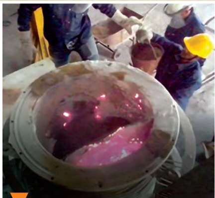
Pyrophoricity of Mg resulted in fire and rapid oxidation
