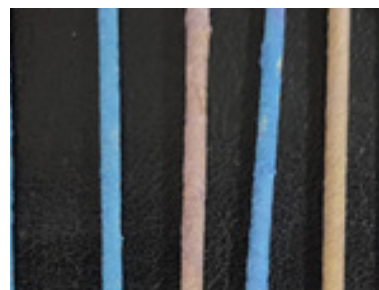
Figure 3: Images of typical silvery-white GI coating along with the colorized surface shades of the hot dip Zn alloy coated steel materials produced at increasing hot dip galvanizing bath temperatures without varying content within less dipping time, followed by normal open-air cooling at room temperature.
