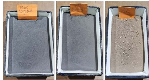
Figure 4: Low-grade iron ore beneficiation products after processing through advanced gravity separation
