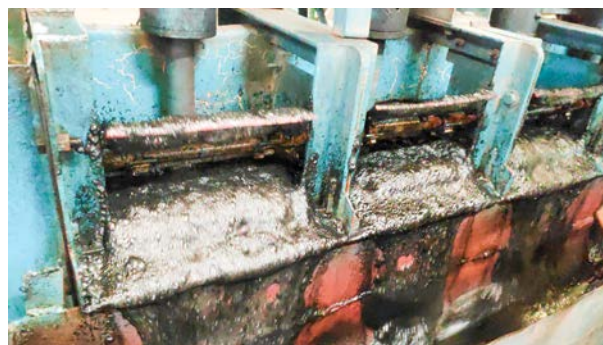
Figure 1: Froth collection during pilot scale flotation trials
