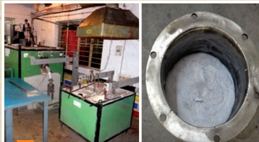
Operation of 500A Sodium Cell & Sodium Collection
