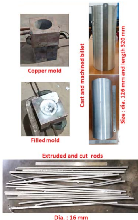
Figure 7: Large scale melting of the alloy to obtain as-cast billet with 140 mm diameter and 330 mm length. The final diameter of the extruded rod was 16 mm
