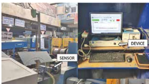
Figure 3: Flaw Guard installed at sponsor's wire mill
