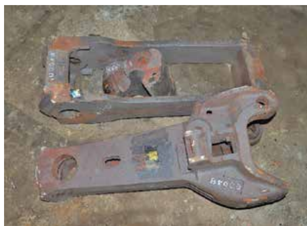
Figure 15: CBC Assembly consisting of body, yoke and knuckle.
