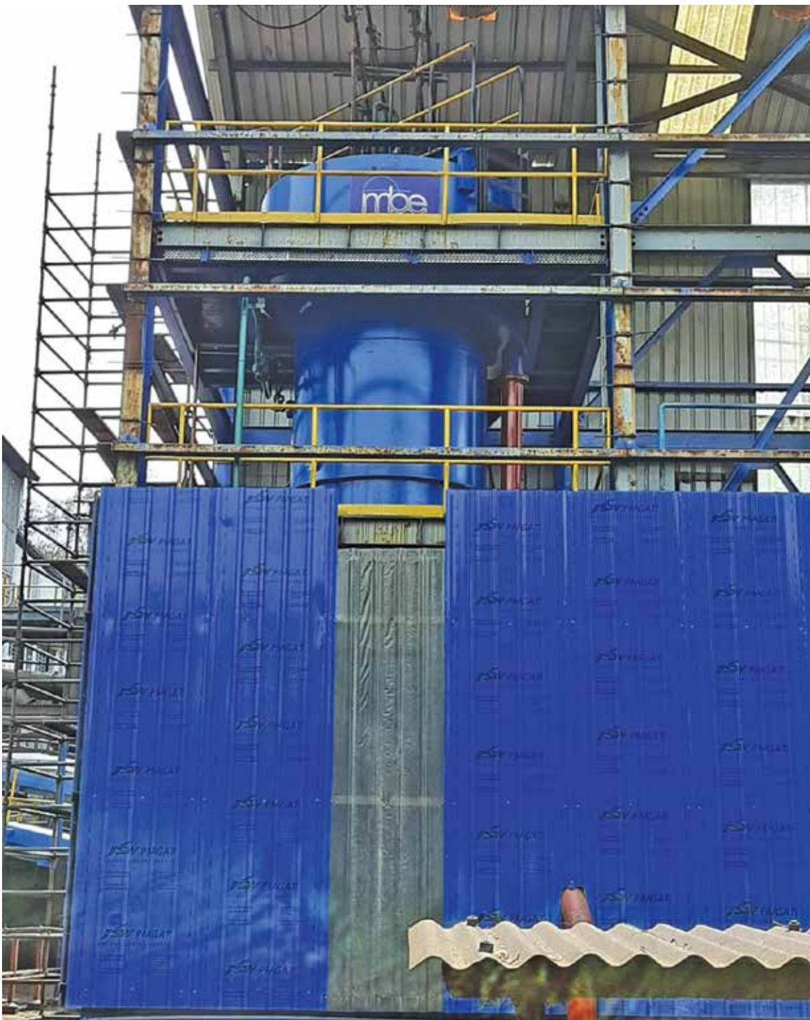
Figure 2: CSIR NML flotation column (2.0m diameter and 9.0m height) in the Coal Preparation Plant
