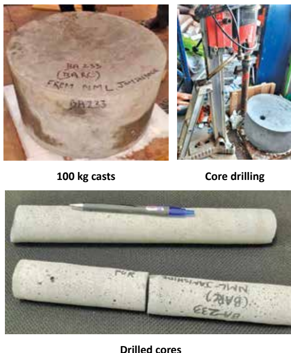
Figure 3: Geopolymerized casts for Immobilization of nuclear wastes, and drilling cores for testing
