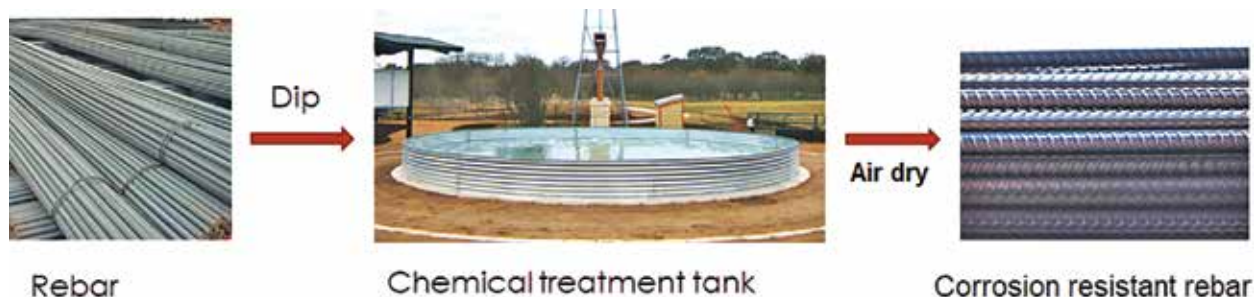
Schematic diagram of rebar chemical treatment process (batch process)
