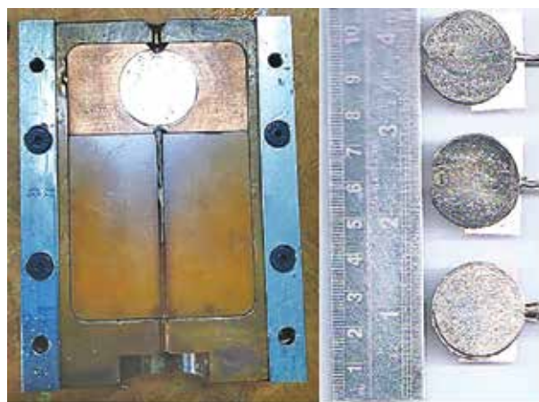
Figure 9: Suction casting mould assembly and 1 mm thick coin samples
