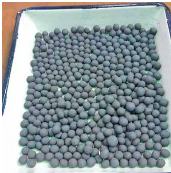
Figure 5: Indurated Iron Ore Pellet Using Organic Binder
