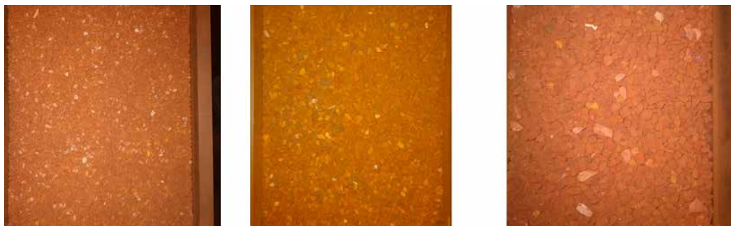
Figure 1: Top-layer after dry processing of iron ore in air pulsated stratifier
