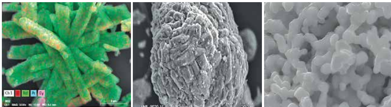
Figure 1: SEM of mixed rare earth oxide, iron oxide and metallic iron powder produced from spent NdFeB magnet
