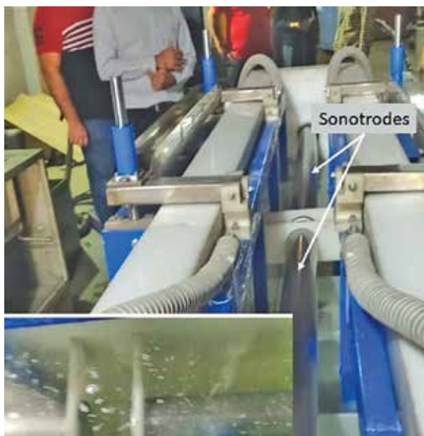
Figure 5: UAET for oxide scale removal of moving wires
