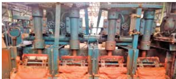
Figure 2: Pilot Scale Processing of Iron Ore Slime
