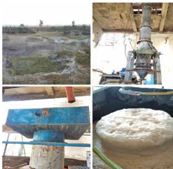
Figure 3: 0.5m diameter Pilot plant scale flotation column
