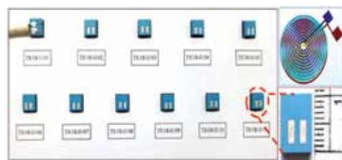
Figure 8 (a): 32 layers' palnar sensor fabricated through LTCC route
