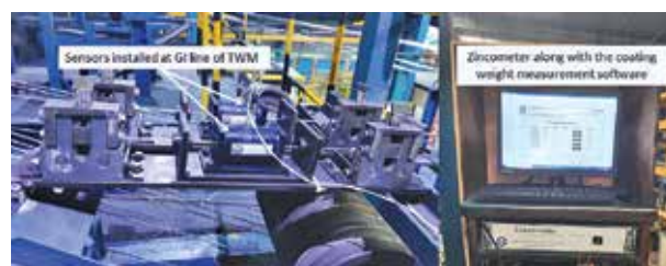
Figure 4: Zincometer installed at sponsor's GI line
