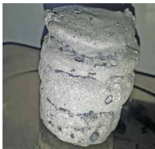
Figure 2: Refined ingot of high purity magnesium containing 99.96-99.97%
