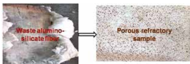
Figure 7: Photograph of clay (alumino-silicate) in combination with Al powder generated porous refractories
