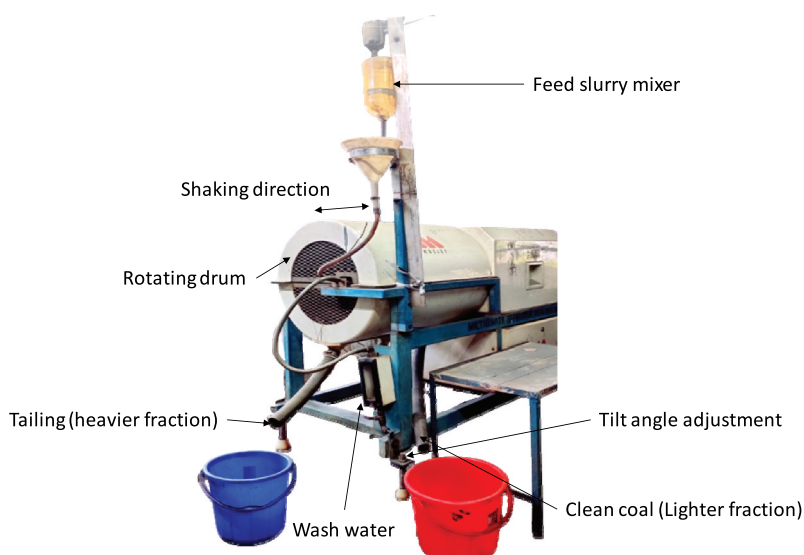
Figure 1. Schematic diagram of C-900 model Mozley Multi Gravity Separator.
