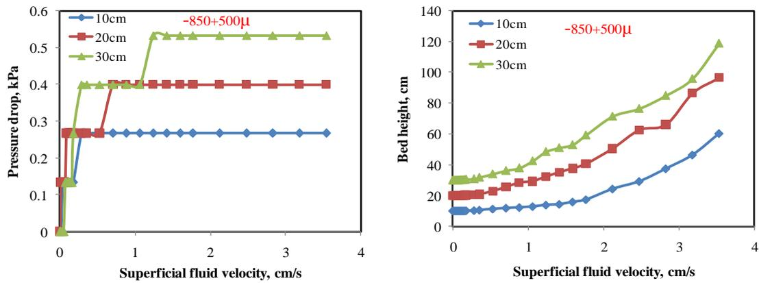
Figure. 6: Pressure drop (left) and bed expansions (right) of coal particles of size -850+500  $\mu$ m at bed heights 10, 20 and 30cm
