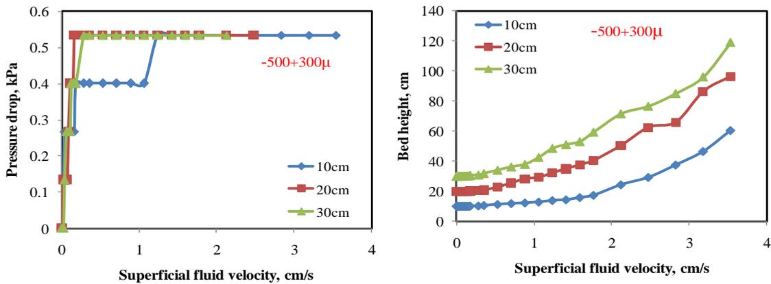
Figure. 7: Pressure drop (left) and bed expansions (right) of coal particles of size -500+300  $\mu$ m at bed heights 10, 20 and 30cm
