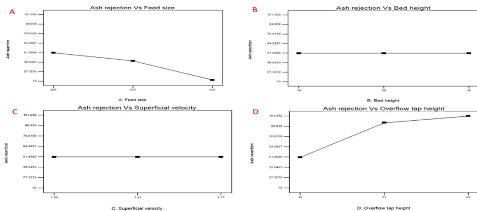
Figure 8: Ash rejection Vs Inputs- A) Feed size, B) Bed height, C) Superficial velocity & D) Overflow tap height
