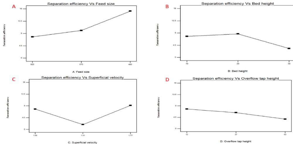
Figure 10: Separation efficiency Vs Inputs- A) Feed size, B) Bed height, C) Superficial velocity & D) Overflow tap height
