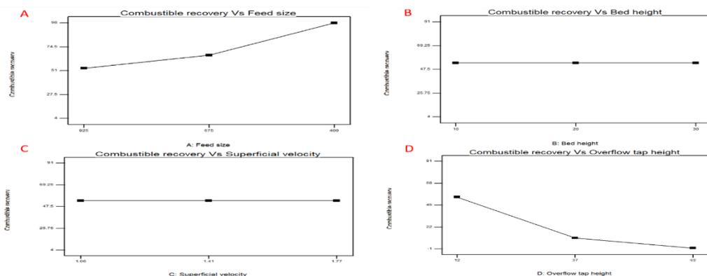
Figure 9: Combustible recovery Vs Inputs- A) Feed size, B) Bed height, C) Superficial velocity & D) Overflow tap height
