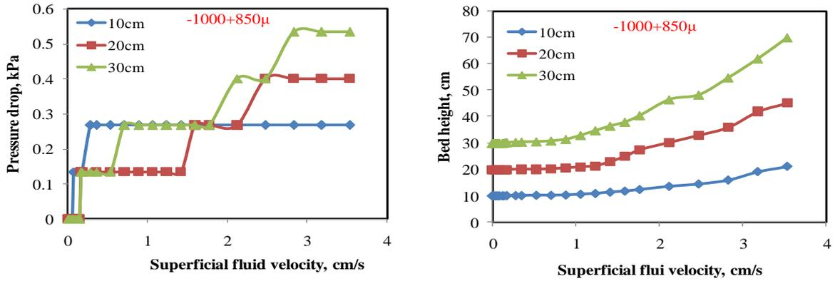
Figure. 5: Pressure drop (left) and bed expansions (right) of coal particles of size -1000+850  $\mu$ m at bed heights 10, 20 and 30cm
