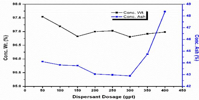
Figure 1: Effect of different dispersant dosage on flocculated concentrates
