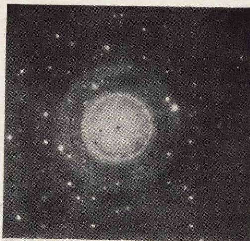
FIG. 25 — ELECTRON DIFFRACTION PATTERN OF THE EXTRACTED RESIDUE OF THE ZONE SHOWN IN FIG. 24
