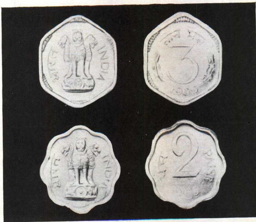
FIG. 34 — THE NEW 2 AND 3 PAISA COINS MADE OF ALUMINIUM-MAGNESIUM ALLOYS DEVELOPED AT NATIONAL METALLURGICAL LABORATORY AND GOVT. OF INDIA MINT, BOMBAY
