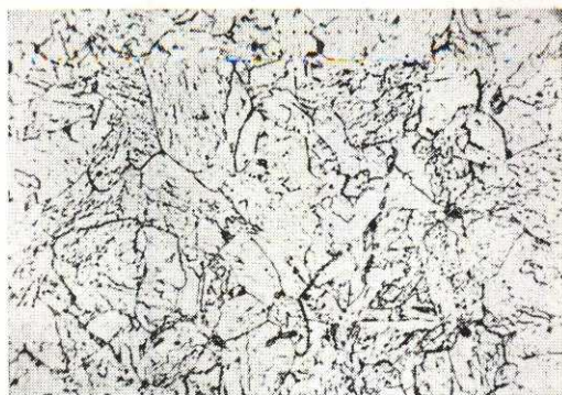
FIG. 26 — MICRO-STRUCTURE OF Nb-TREATED STEEL D. NORMALIZED AT 950°C \times 470 NITAL ETCHED
