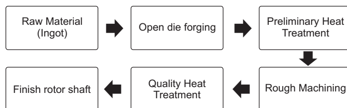
Fig. 2 : Flow chart of rotor shaft
