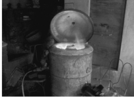
Fig. 10.8 : Photograph of the Developed Furnace indicating burner in action
