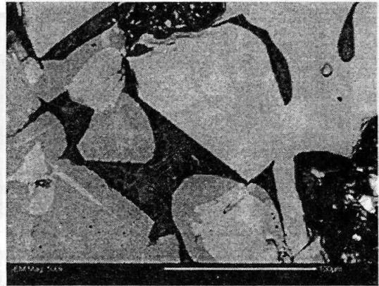
Fig. 4: Back Scattered Electron Image of Sintered Pellets of + 150 Kg Strength
