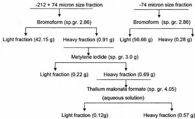
**Fig. 1: Scheme and Results of Heavy Liquid Test of Bauxite Sample**
