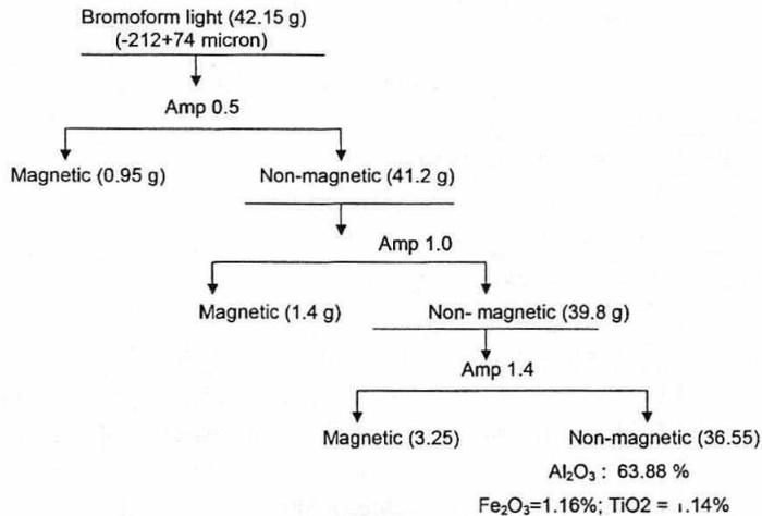
**Fig. 2: Result of Isodynamic Test on -212+74 Micron Size Fraction**
