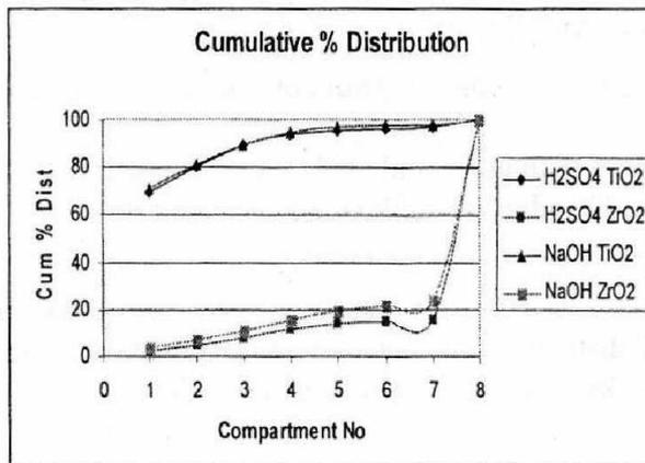
**Fig. 6: Cumulative Distribution of TiO<sub>2</sub> and ZrO<sub>2</sub> in Electrostatic Separation**
