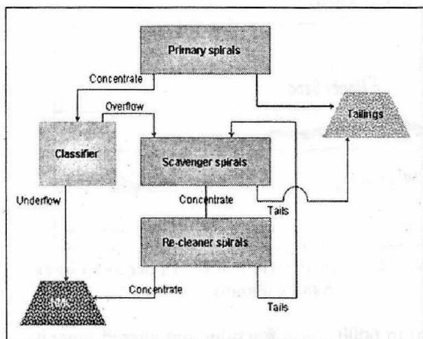
**Fig. 3: Normal All Spiral Flow Sheet used for Primary Concentration**
