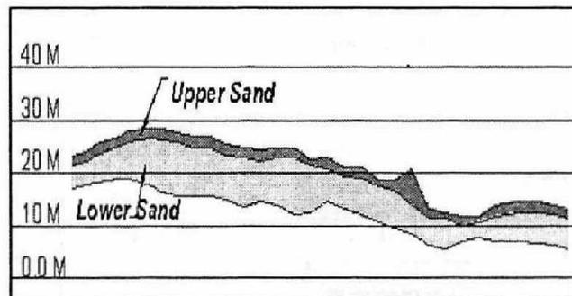
Fig. 2: Typical Geological Section of the Upper and Lower Sand Columns
