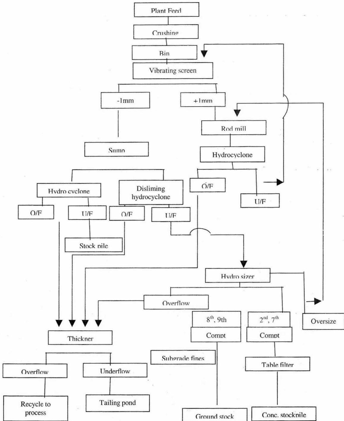
**Fig 1. Flowsheet of a Chromite Ore Beneficiation Plant**
