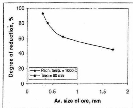
Fig. 3.3 : Effect of size of ore on degree of reduction.
