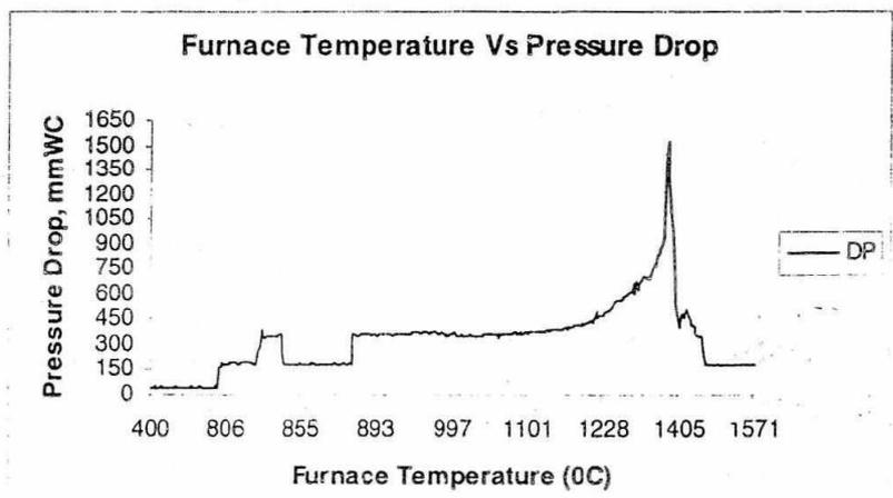
Fig. 3.9: Drop in pressure with furnace temperature during softening– melting experiment
