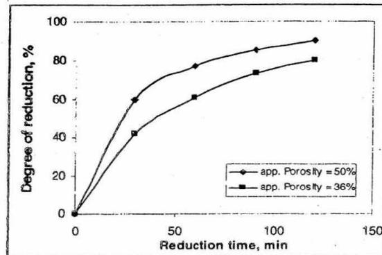
Fig. 3.7 : variation of degree of reduction with reduction time for pellets having different porosity
