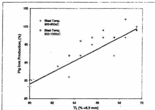
Fig. 3.4 : Effect of tumbler index of sinter on blast furnace productivity
