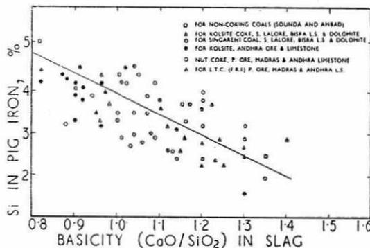
9 The effect of basicity on silicon contents of pig iron
