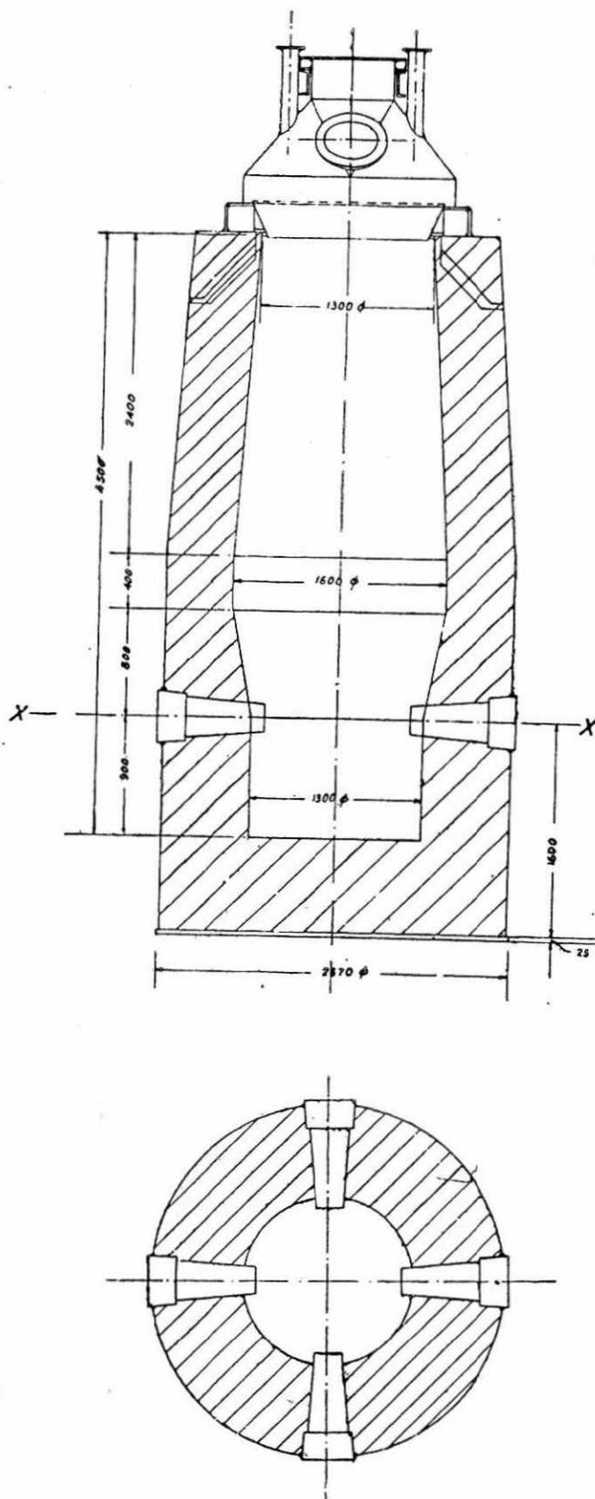
1 Section through shaft and hearth of the 15 tonnes/day low shaft furnace
