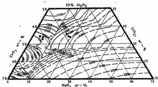
12 Liquidus temperature of CaO-SiO<sub>2</sub>-MgO slags at 20% Al<sub>2</sub>O<sub>3</sub> level
