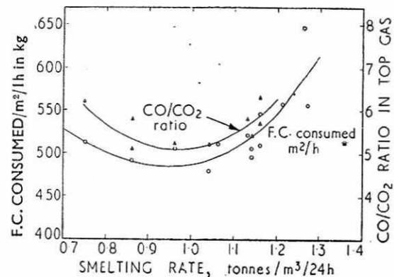
15 Dependence of fuel rate on smelting rate
