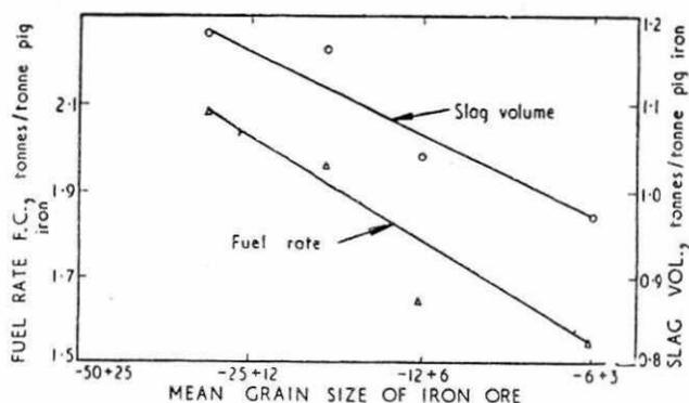
13 Variation of fuel rate and slag volume with particle size of iron ore
