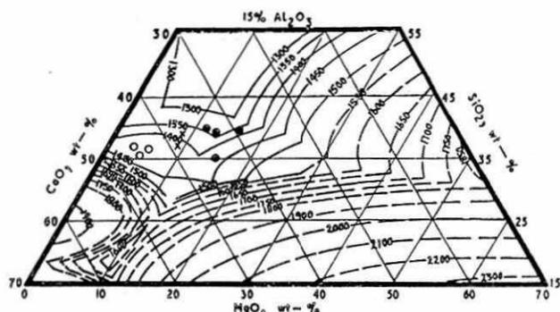
11 Liquidus temperature CaO-SiO<sub>2</sub>-MgO slags at 15% Al<sub>2</sub>O<sub>3</sub> level
