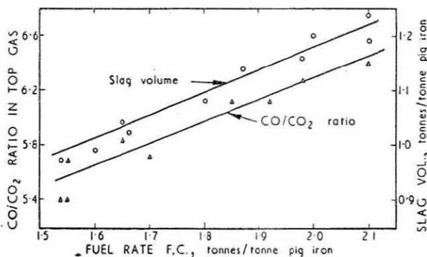
14 Variation of fuel rate and slag volume with CO/CO<sub>2</sub> ratio
