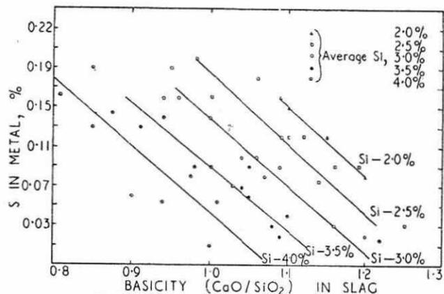
8 Effects of silicon and basicity ratios on the partition of sulphur
