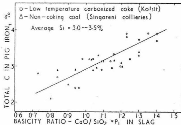
10 Dependence of carbon contents of pig iron on basicity ratio
