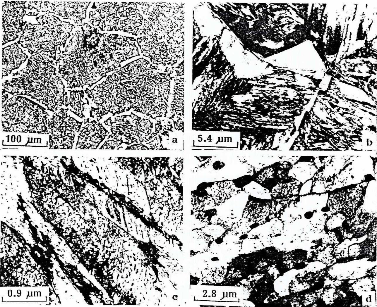
Fig.3. (a)-(c) Microstructures of Forged + water quenched (FQ) and (d) Forged + water quenched + tempered at 675 °C for 52 hrs. (FOT), HSLA steel. Fig. (a) is the optical micrograph showing thick ferrite along the prior austenite grain boundaries. Figs. (b) and (c) are the TEM micrographs showing slabs of ferrite precipitation, lath martensite and acicular ferrite. Fig.(d) shows spheroidisation of carbides and polygonisation of ferrites.
